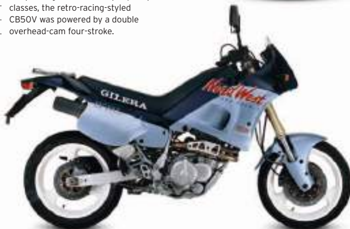
▷ Gilera Nord West 600 1991 Origin Italy Engine 556 cc, single-cylinder Top speed 106 mph (170 km/h)
