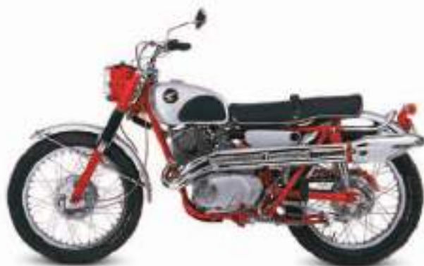
△ Honda CL72 Scrambler 1964 Origin Japan Engine 247 cc, in-line two Top speed 75 mph (120 km/h)
