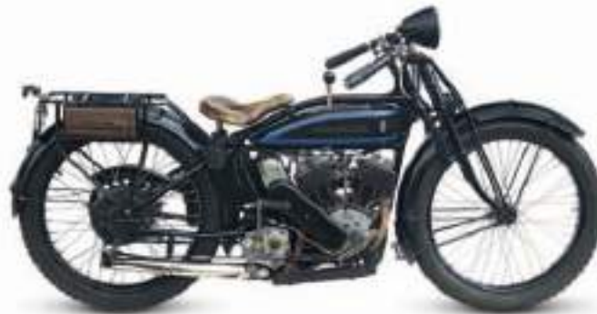
◁ Husqvarna T180 1926 Origin Sweden Engine 550 cc, V-twin Top speed 60 mph (97 km/h)
