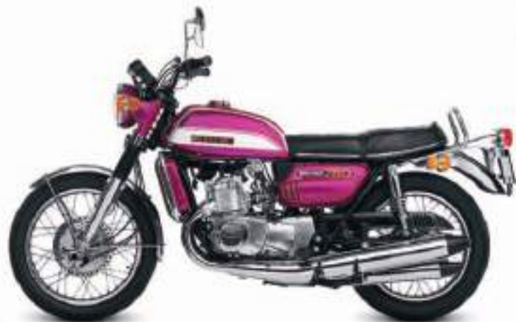
△ Suzuki GT750 1978 Origin Japan Engine 738 cc, in-line triple Top speed 123 mph (198 km/h)
