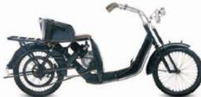
◁ DKW Lomos 1922 Origin Germany Engine 143 cc, single-cylinder Top speed 37 mph (60 km/h)
