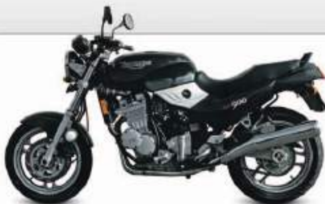
◁ Triumph Trident 900 1990 Origin UK Engine 885 cc, in-line triple Top speed 133 mph (214 km/h)
