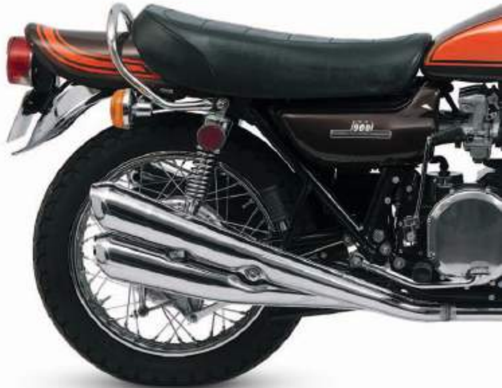
△ Kawasaki Z1 1973 Origin Japan Engine 903 cc, in-line four Top speed 135 mph (217 km/h)
