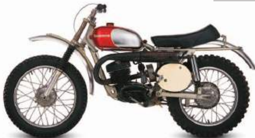
△ Husqvarna 250 1963 Origin Sweden Engine 250 cc, single-cylinder Top speed 75 mph (120 km/h)
