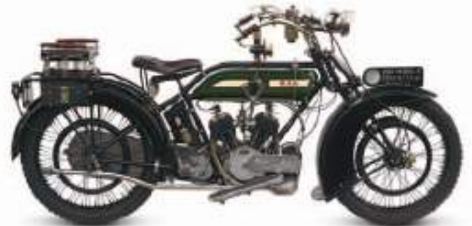
▷ BSA Model A 1922 Origin UK Engine 770 cc, V-twin Top speed 55 mph (89 km/h)
