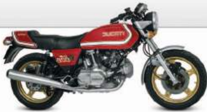
◁ Ducati 900SD Darmah 1979 Origin Italy Engine 864 cc, V-twin Top speed 114mph (183 km/h)
