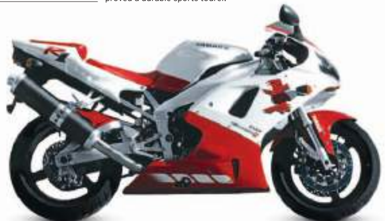
△ Yamaha YZF-R1 1998 Origin Japan Engine 998 cc, in-line four Top speed 171 mph (275 km/h)
