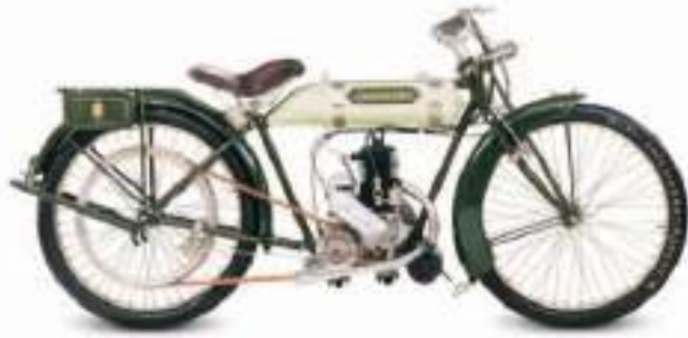
△ Triumph Knirps 2 1/2 HP 1920 Origin Germany Engine 276 cc, single-cylinder Top speed 52 mph (84 km/h)
