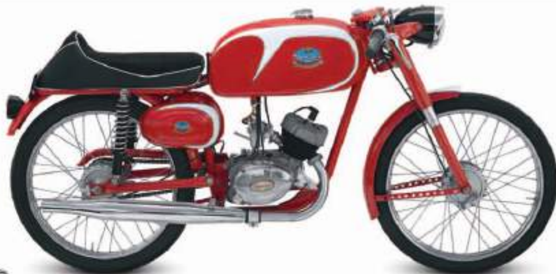
△ FB Mondial 48 Sport 1960 Mondial's racy 50 cc model was aimed at enthusiastic young riders. This type of machine's popularity was reflected by the 1962 launch of a 50 cc Grand Prix class. Origin Italy Engine 48 cc, single-cylinder Top speed 45 mph (72 km/h)
