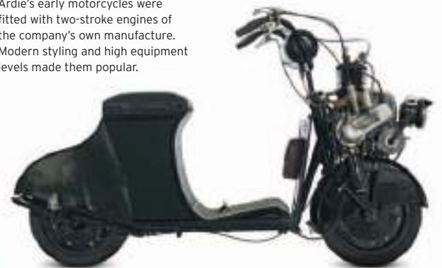
△ Autoglider Model D 1921 Origin UK Engine 269 cc, single-cylinder Top speed 45 mph (72 km/h)
