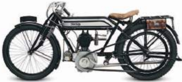
△ Norton Model 9 1920 Origin UK Engine 490 cc, single-cylinder Top speed 70 mph (113 km/h) The Model 9's side-valve engine dated back to James Lansdowne Norton's first engine of 1908. It was flexible and powerful but outdated, with no clutch or gears.
