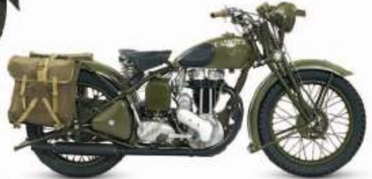
Origin UK Engine 347 cc, ohv single-cylinder Top speed 65 mph (105 km/h)
