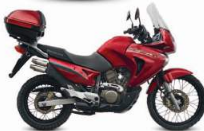
△ Honda Transalp XL650V-6 2007 Origin Japan Engine 647cc, V-twin Top speed 105mph (169km/h)
