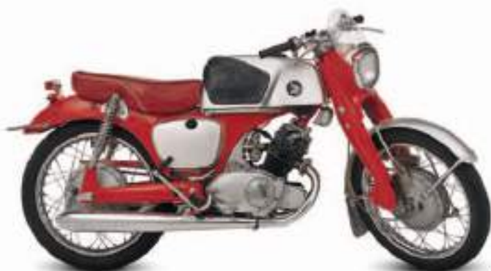
△ Honda CB92 Benly Super Sports 1961 The fastest 125 of its day, this model was a great standard bearer for Japan's motorcycling industry. The little CB92's ruggedly made overhead-camshaft engine revved to more than 10,000 rpm. Origin Japan Engine 124 cc, in-line two Top speed 70 mph (113 km/h)
