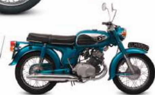
◁ Honda CD175 1967 Origin Japan Engine 174 cc, in-line two Top speed 78 mph (126 km/h)
