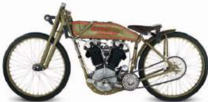
△ Harley-Davidson Eight-valve Racer 1920 Origin USA Engine 1,000 cc, V-twin Top speed 120 mph (193 km/h)
