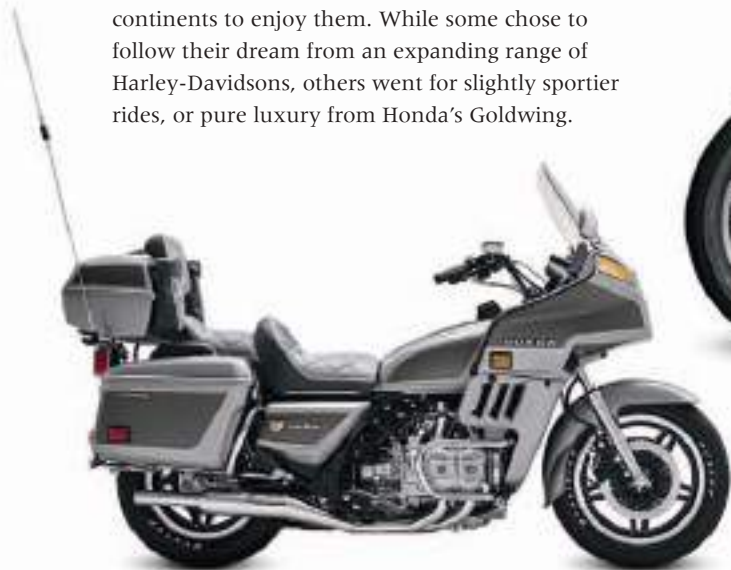
△ Honda GL1100 Goldwing Aspencade 1982 Origin Japan Engine 1,085 cc, flat-four Top speed 103 mph (166 km/h)
