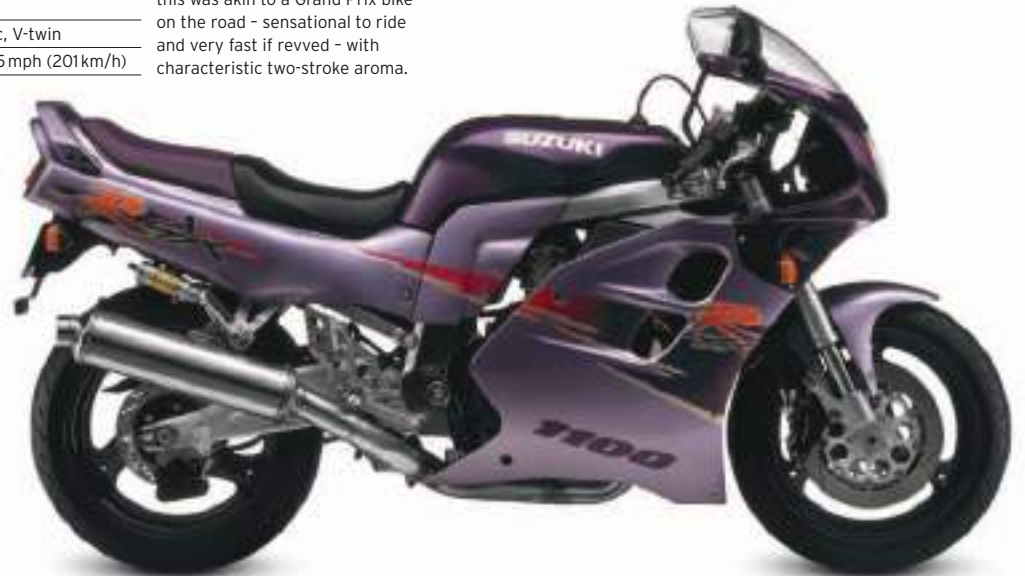
△ Suzuki GSX-R1100 1994 Origin Japan Engine 1,074 cc, in-line four Top speed 169 mph (272 km/h)
