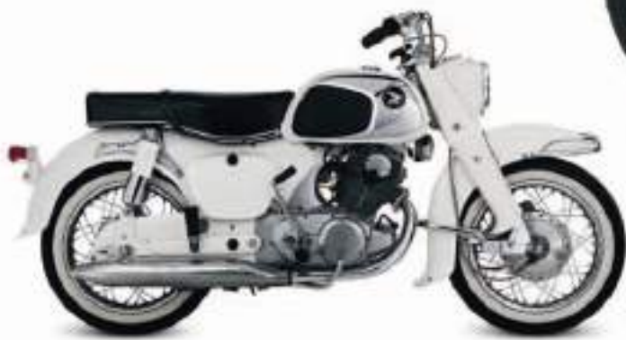
△ Honda C77 Dream 300 1961 First released in 1956 but redesigned for 1960, the Dream was a high-specification, well-equipped bike that looked rather expensive alongside more basic machines. Origin Japan Engine 305 cc, in-line two Top speed 88 mph (142 km/h)
