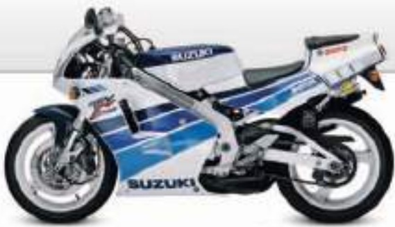
◁ Suzuki RGV 250 1990 Origin Japan Engine 249 cc, V-twin Top speed 125 mph (201km/h)
