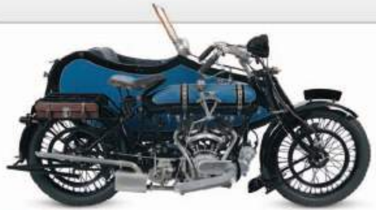
△ Martinsyde 680 Combination 1921 Origin UK Engine 677 cc, V-twin Top speed 58 mph (93 km/h)
