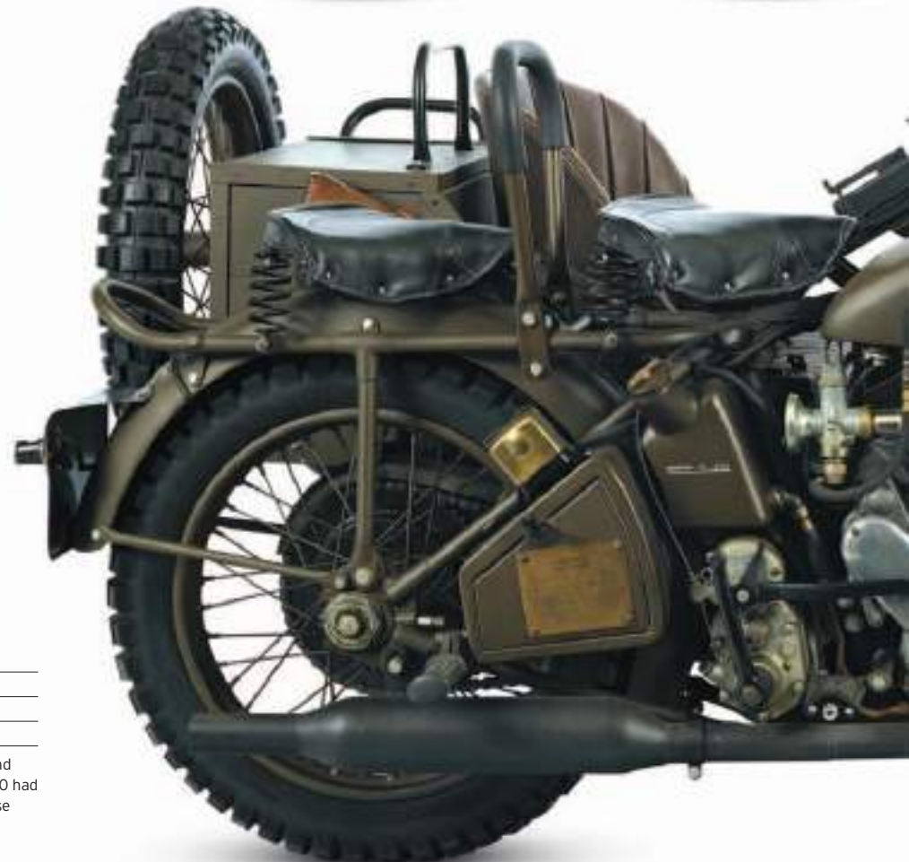
Origin Germany Engine 751 cc, ohv flat-twin Top speed 60 mph (97 km/h)
