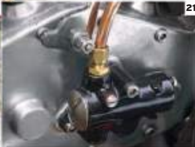
15. 750cc engine 16. Battery box 17. Side view of engine showing V-twin cylinders 18. Magneto and dynamo 19. Choke lever on carburettor 20. Fuel tap 21. External oil pump 22. Fuel priming cup
