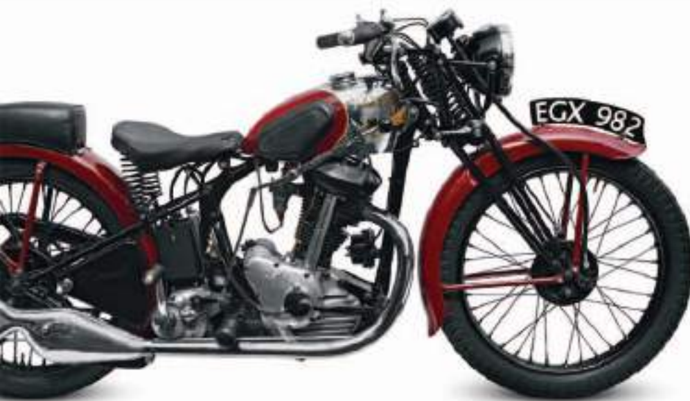
△ Panther 250 Red Panther 1932 Unlike Panther's bigger singles, the 250 did not use the cylinder in place of a frame downtube. It was the UK's cheapest machine in its class.
