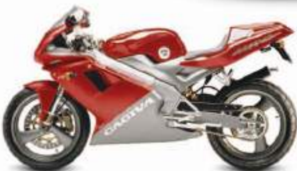
△ Cagiva Mito 125 Evoluzione 1994 Origin Italy Engine 126 cc, single-cylinder Top speed 107 mph (172 km/h)
