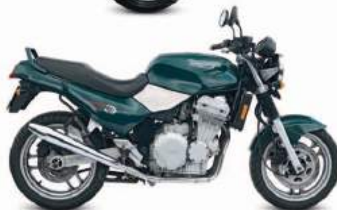
△ Triumph Trident 750 1991 Origin UK Engine 749 cc, in-line three Top speed 134 mph (216 km/h) With easily enough power to be fun and a relatively upright driving position ideal for town and traffic riding, the water-cooled 750 was a welcome addition to the Triumph range.
