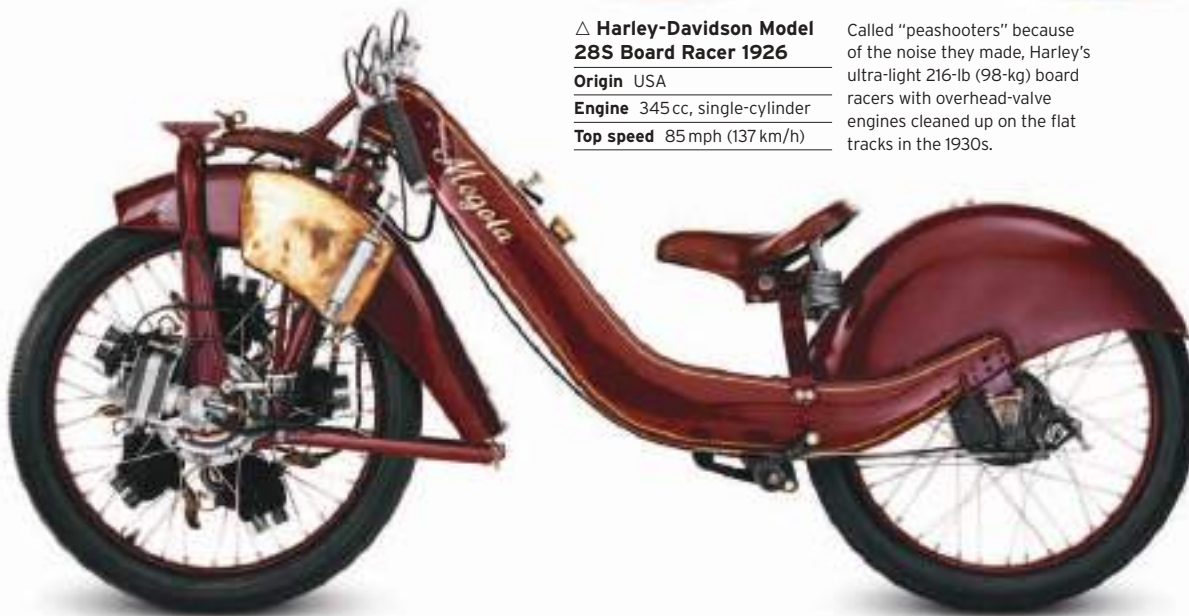
◁ Megola 1921 1923 Origin Germany Engine 640 cc, rotary five-cylinder Top speed 88 mph (142 km/h)
