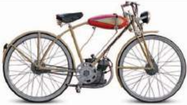
△ Ducati Cucciolo 1949 Origin Italy Engine 48 cc, single-cylinder Top speed 40 mph (64 km/h)
