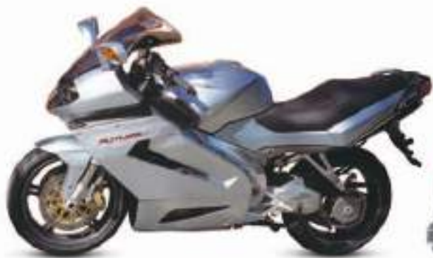
△ Aprilia RST Futura 2001 Origin Italy Engine 998cc, V-twin Top speed 150mph (241km/h)
