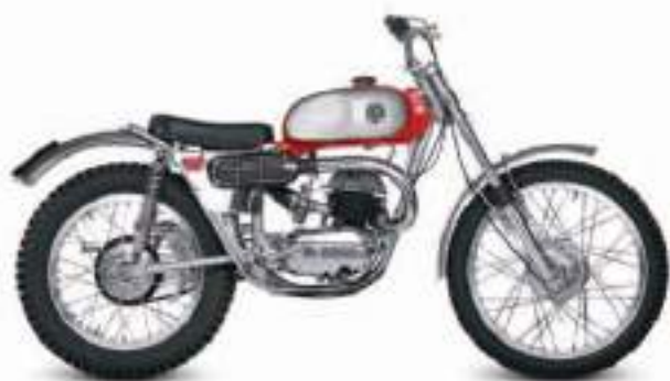
△ Bultaco Sherpa T 1964 Origin Spain Engine 244 cc, single-cylinder Top speed 75 mph (120 km/h)
