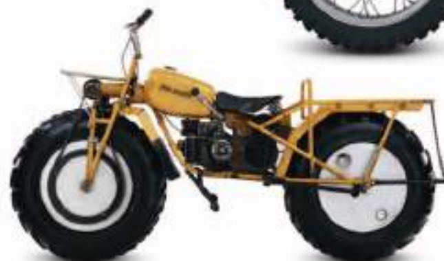
△ Rokon Trail-breaker 1963 Origin USA Engine 134 cc, single-cylinder Top speed 20 mph (32 km/h)
