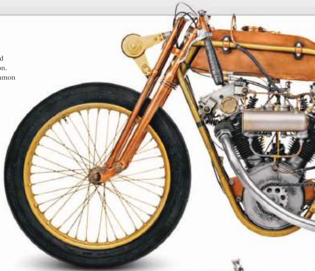
▷ Indian Model H 1920 Origin USA Engine 1,000 cc, V-twin Top speed 120 mph (193 km/h)
