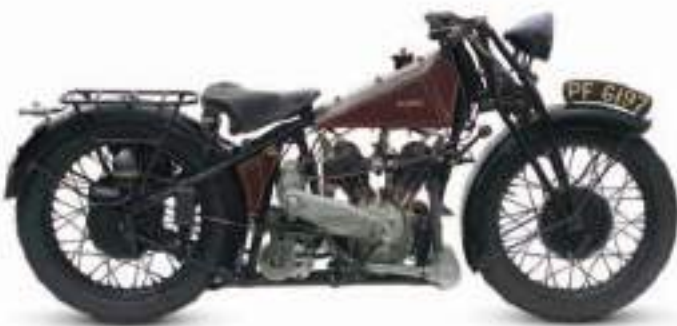
▷ Coventry-Eagle Flying 8 1925 Origin UK Engine 980 cc, V-twin Top speed 100 mph (160 km/h)
