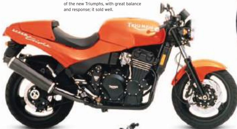
▽ Triumph Speed Triple 1994 Origin UK Engine 885 cc, in-line triple Top speed 135 mph (217 km/h)
