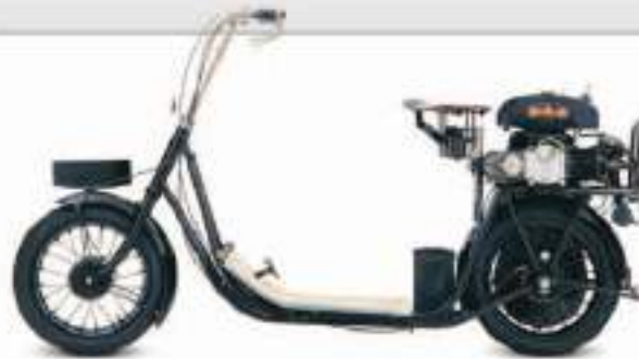
◁ ABC Skootamota 1920 Origin UK Engine 123 cc, single-cylinder Top speed 15 mph (24 km/h)
