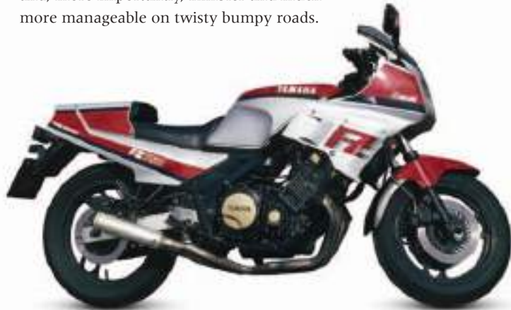
△ Yamaha FZ750 1985 Origin Japan Engine 749 cc, in-line four Top speed 145 mph (233 km/h)
