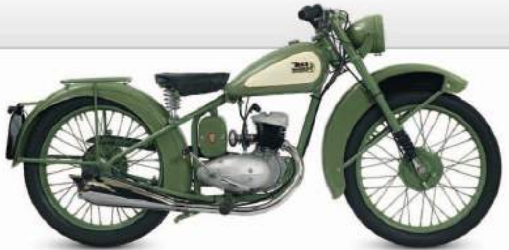
△ BSA Bantam D1 1949 Origin UK Engine 123 cc, single-cylinder Top speed 53 mph (85 km/h)
