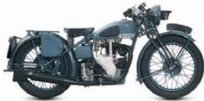
△ Velocette MAC-MDD 1940 Origin UK Engine 349 cc, ohv single-cylinder Top speed 75 mph (120 km/h)
