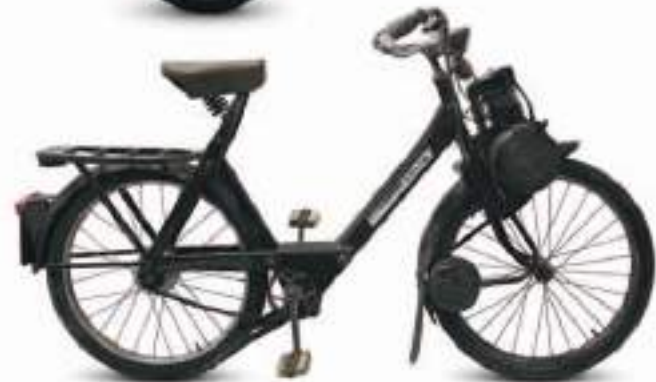
△ VéloSoleX 45 1949 Origin France Engine 45 cc, single-cylinder Top speed 21 mph (34 km/h)
