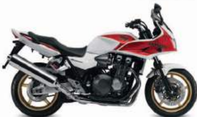
△ Honda CB1300 2012 Origin Japan Engine 1,284 cc, in-line four Top speed 136 mph (219 km/h)
