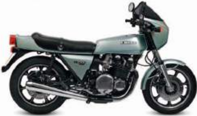
△ Kawasaki Z1000 Z1R D1 1978 Origin Japan Engine 1,015 cc, in-line four Top speed 136mph (219 km/h)
