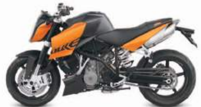
▷ KTM 990 Super Duke 2011 Origin Austria Engine 999 cc, V-twin Top speed 151 mph (243 km/h)
