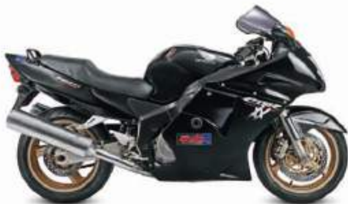
△ Honda CBR1100XX Super Blackbird 2002 Origin Japan Engine 1,137cc, in-line four Top speed 188mph (303km/h)
