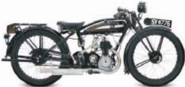
△ Triumph Model W 1927 Origin UK Engine 277 cc, single-cylinder Top speed 48 mph (77 km/h)
