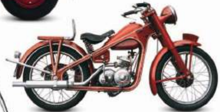
△ Honda Model D Dream 1949 Origin Japan Engine 98 cc, single-cylinder Top speed 40 mph (64 km/h)
