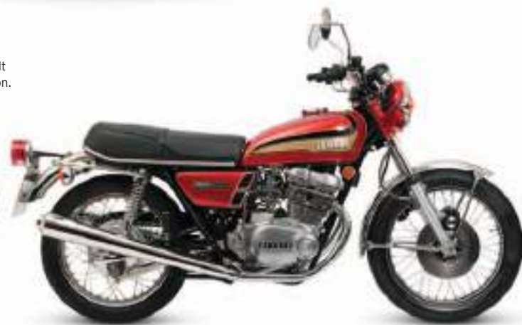
△ Yamaha TX500 1972 This was the first road bike to combine double overhead camshafts and four valves per cylinder on a parallel-twin. It was docile and civilized to ride.
