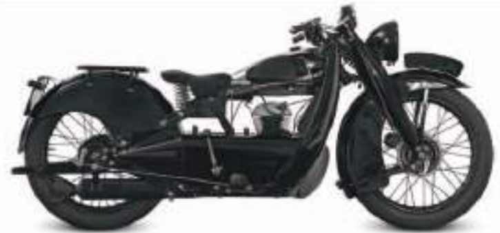
△ Francis-Barnett Cruiser 1933 Aimed at non-enthusiast buyers looking for a more convenient alternative to the bus, the Cruiser's pressed-steel bodywork offered good weather protection.
