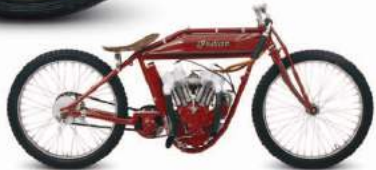
▷ Indian Model H 1920 Origin USA Engine 1,000 cc, V-twin Top speed 120 mph (193 km/h)
