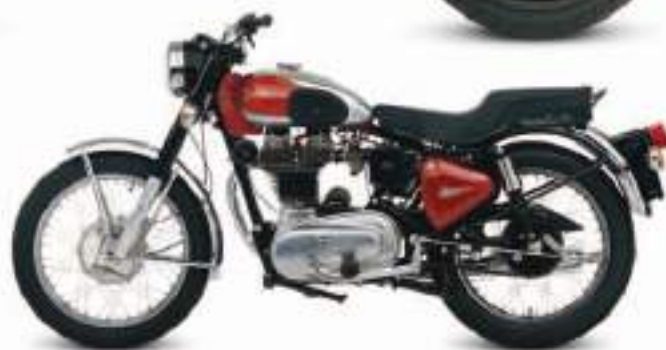
△ Enfield India Bullet 350 1992 Origin India Engine 346 cc, single-cylinder Top speed 68 mph (109 km/h) The Bullet has been built in India since 1955, and with minimal upgrades. It still has the same period charm of the original British-built machines.
