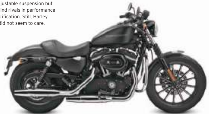
△ Harley-Davidson Sportster XL883N Iron 2011 Origin USA Engine 883 cc, V-twin Top speed 105 mph (169 km/h)
