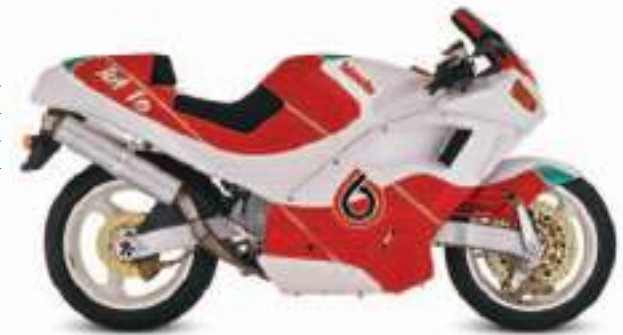
▷ Bimota Tesi 1D 906 1992 Origin Italy Engine 904 cc, V-twin Top speed 155 mph (249 km/h)
