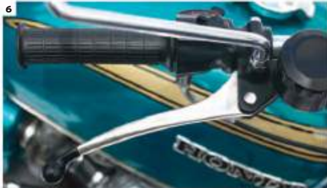
1. Tank script 2. Fork gaiters 3. Side reflector 4. Honda wing badge on side panel 5. Handlebar switchgear 6. Front brake lever 7. Front brake disc 8. Rear shock 9. 140mph (225km/h) speedometer 10. Passenger footrest 11. Kick-starter provides back-up 12. Front wheel hub cone 13. Exhaust outlets
