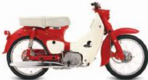
△ Honda Juno M85 1962 Only made for one year the Juno was an innovative steel monocoque scooter with an exposed flat-twin engine and variable hydraulic mechanical transmission. Origin Japan Engine 169 cc, flat-twin Top speed 62 mph (100 km/h)
