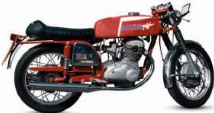
△ MV Agusta 350S Elettronica 1972 This bike had excellent handling thanks to a lightweight frame that incorporated the engine as a structural member. The 1972 model was equipped with an early form of electronic ignition.
