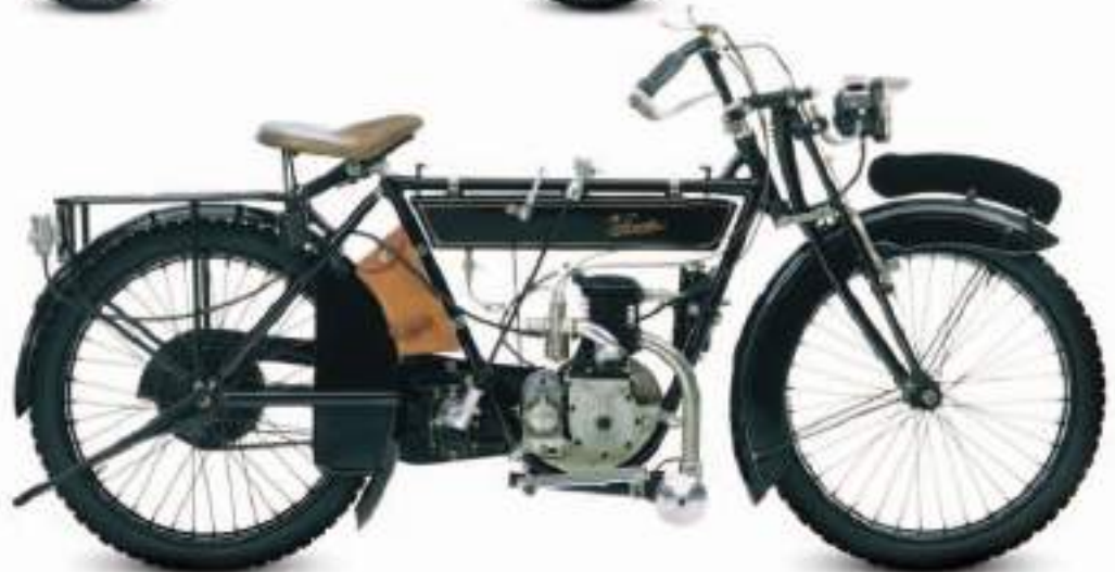
◁ Ardie 3PS 1922 Origin Germany Engine 304 cc, single-cylinder Top speed 52 mph (84 km/h)
