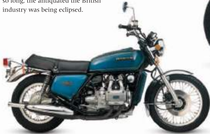
△ Honda Goldwing GL1000 1975 Advanced automotive technology made the Goldwing a sophisticated, powerful, and heavy machine that became the definitive touring motorcycle. Origin Japan Engine 999 cc, flat-four Top speed 125 mph (201 km/h)
