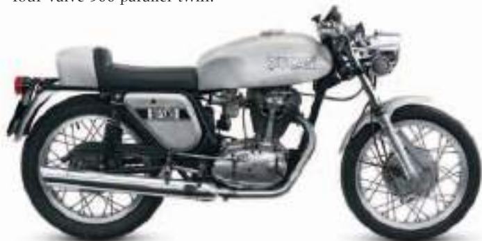
△ Ducati Silver Shotgun 1970 With its glassfibre café-racer body panels painted in silver metalflake, you could not miss this Ducati, nor the sound of its desmodromic engine revving at 7,000 rpm.
