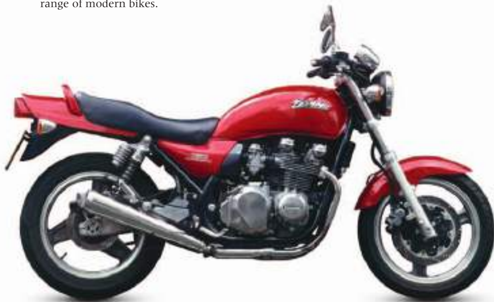
△ Kawasaki 750 Zephyr 1990 Origin Japan Engine 738 cc, in-line four Top speed 126 mph (203 km/h) Blending 1970s styling with modern detail such as three-spoke alloy wheels, good brakes and suspension, plus a competitive price, brought Kawasaki another winner in the 750 Zephyr.
