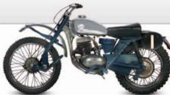
△ Greeves Hawkstone 1961 Origin UK Engine 249 cc, in-line two Top speed 70 mph (113 km/h)
