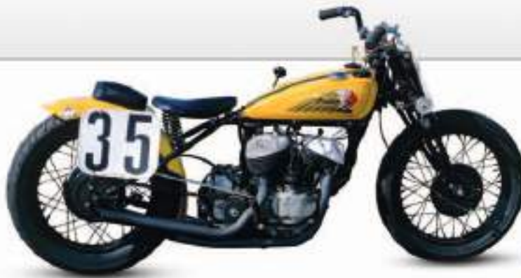
△ Indian Sport Scout 1936 Origin USA Engine 737 cc, side-valve V-twin Top speed 85 mph (137 km/h)
