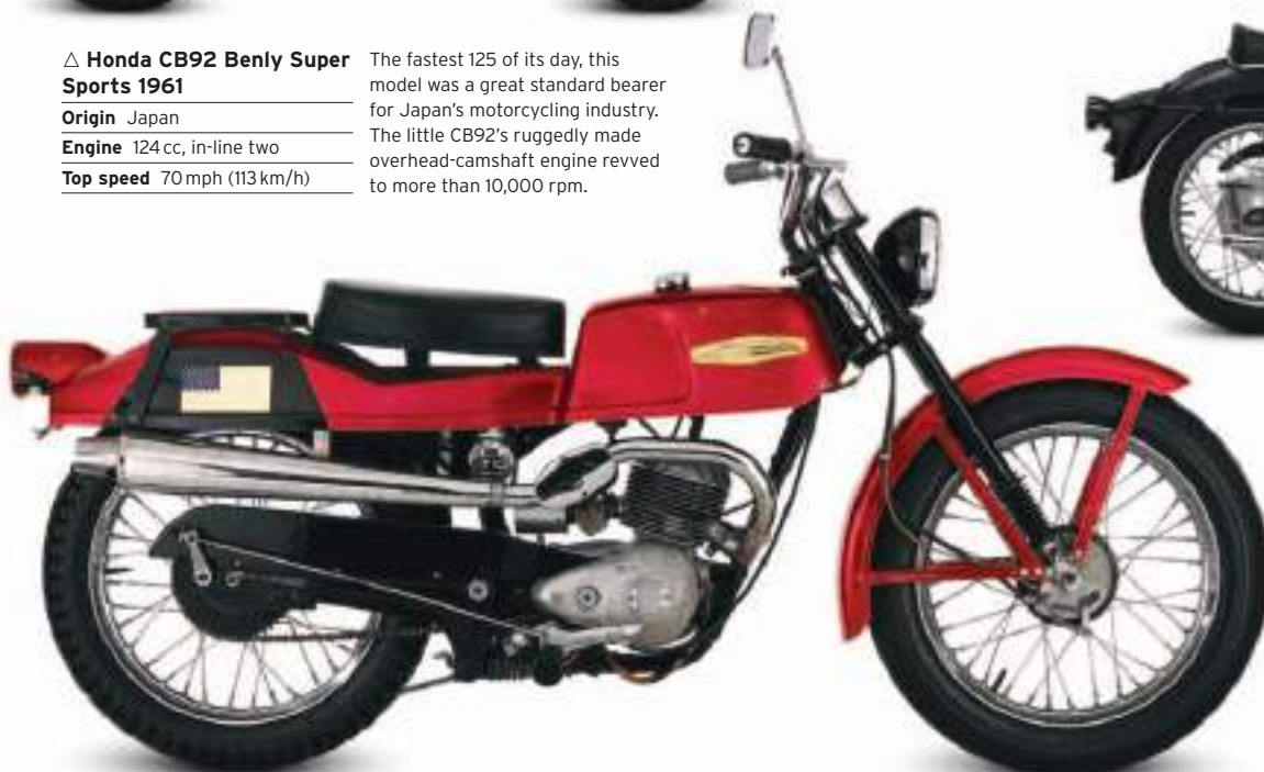
△ Harley-Davidson Sprint H 1962 Made in Italy by Aermacchi, the Sprint singles filled the gap in Harley's model line that was being exploited by Japanese imports. A 350 cc bike was introduced for 1969. Origin USA/Italy Engine 246 cc, single-cylinder Top speed 76 mph (122 km/h)
