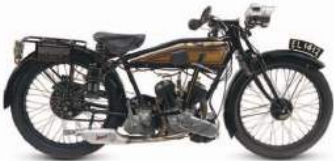
△ James Model 12 1925 Origin UK Engine 495 cc, V-twin Top speed 53 mph (85 km/h)
