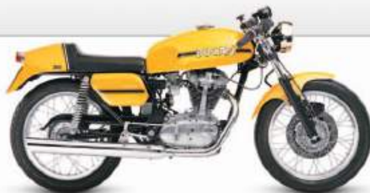
△ Ducati 350 Desmo 1974 Fabio Tagliani devised a desmodromic system that opened and closed the valves without springs, to give these singles an exceptionally high performance.
