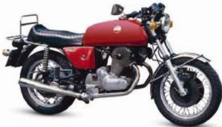
△ Laverda 750SF2 1972 Laverda's first large-capacity bikes were sturdily built overhead-camshaft twins with inclined cylinders. The SF sport versions handled well and were successful in Endurance races. Origin Italy Engine 744 cc, ohc parallel-twin Top speed 118 mph (190 km/h)
