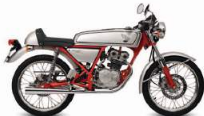
△ Honda CB50V Dream 1996 Origin Japan Engine 49 cc, single-cylinder Top speed 50 mph (80 km/h) Conceived to commemorate Honda's early racing success in tiny capacity classes, the retro-racing-styled CB50V was powered by a double overhead-cam four-stroke.
