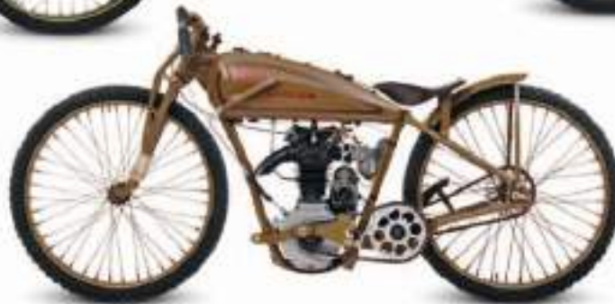
△ Harley-Davidson Model 28S Board Racer 1926 Origin USA Engine 345 cc, single-cylinder Top speed 85 mph (137 km/h)
