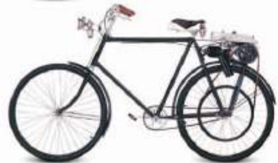
◁ DKW Lomos 1922 Origin Germany Engine 143 cc, single-cylinder Top speed 37 mph (60 km/h)
