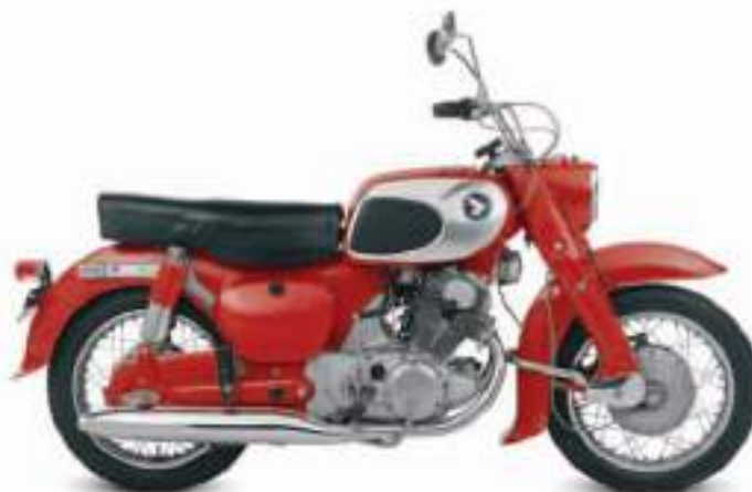
△ Honda CB72 Dream 1961 Honda favoured pressed-steel frames that used the power unit as a stressed member, leading link front forks, and styling that looked slightly odd to Western eyes. Noted for its quality engineering, this model sold well. Origin Japan Engine 247 cc, in-line two Top speed 80 mph (129 km/h)
