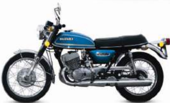
△ Suzuki T500 1975 This first two-stroke to win an AMA National race was also the world's largest two-stroke twin at the time, prone to vibration but worth it for the performance on offer. Origin Japan Engine 492 cc, in-line twin Top speed 106 mph (170 km/h)
