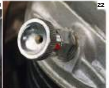
15. 750cc engine 16. Battery box 17. Side view of engine showing V-twin cylinders 18. Magneto and dynamo 19. Choke lever on carburettor 20. Fuel tap 21. External oil pump 22. Fuel priming cup
