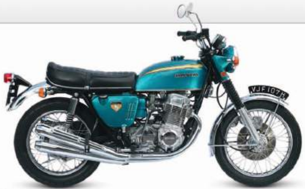
△ Honda CB750 1970 This was the first superbike: Honda changed the face of sports bikes in 1969 with its overhead-camshaft four-cylinder engine, disc brake, and refined details. Origin Japan Engine 736 cc, in-line four Top speed 125 mph (201 km/h)
