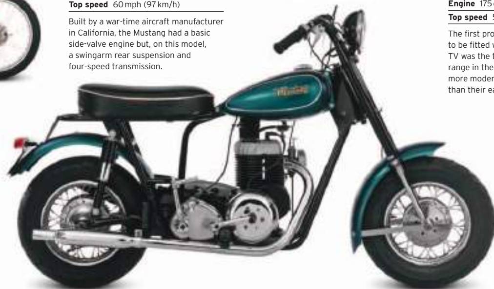
▽ Mustang Thoroughbred 1962 Origin USA Engine 320 cc, single-cylinder Top speed 60 mph (97 km/h)
