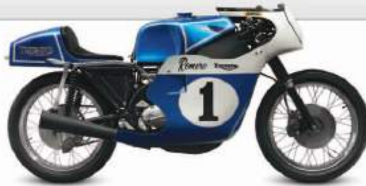
◁ Triumph F750 1971 Origin UK Engine 741 cc, in-line twin Top speed 140 mph (225 km/h)
