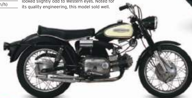
△ Harley-Davidson Sprint H 1962 Made in Italy by Aermacchi, the Sprint singles filled the gap in Harley's model line that was being exploited by Japanese imports. A 350 cc bike was introduced for 1969. Origin USA/Italy Engine 246 cc, single-cylinder Top speed 76 mph (122 km/h)
