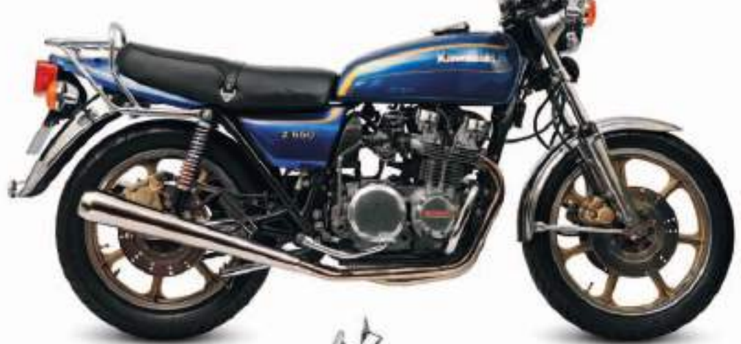
△ Kawasaki Z650C 1979 Origin Japan Engine 652 cc, in-line four Top speed 118mph (190 km/h)
