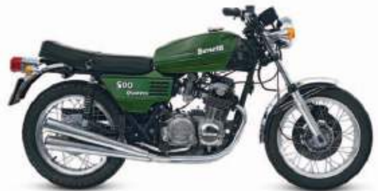
△ Benelli 500 Quattro 1975 Under De Tomaso's control, Benelli's Honda-like engine was built by Moto Guzzi. With a disc front brake, good power output, and excellent economy, this was an attractive bike. Origin Italy Engine 498 cc, in-line four Top speed 107 mph (172 km/h)
