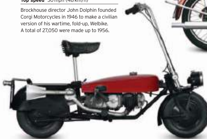
▽ Brockhouse Corgi 1949 Origin UK Engine 98 cc, single-cylinder Top speed 30 mph (48 km/h)
