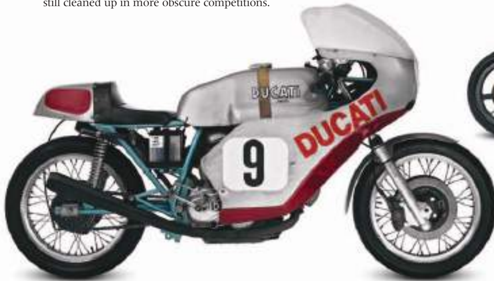
△ Ducati 750SS 1972 Origin Italy Engine 748 cc, V-twin Top speed 140 mph (225 km/h)
