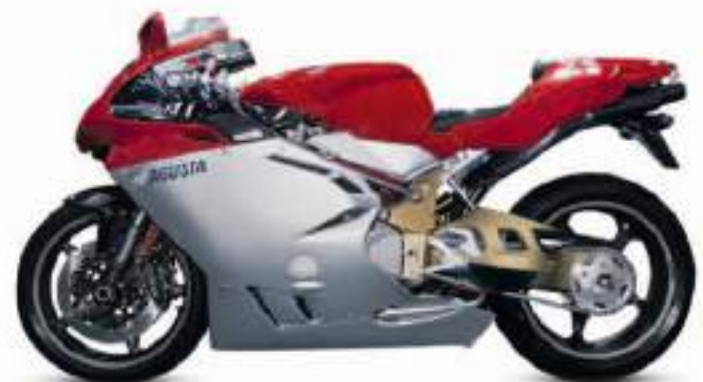
△ MV Agusta F4 750S 1999 Origin Italy Engine 749 cc, in-line four Top speed 175 mph (282 km/h)
