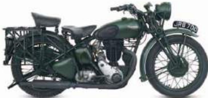
△ Triumph 3HW 1944 Origin UK Engine 343 cc, ohv single-cylinder Top speed 65 mph (105 km/h)
