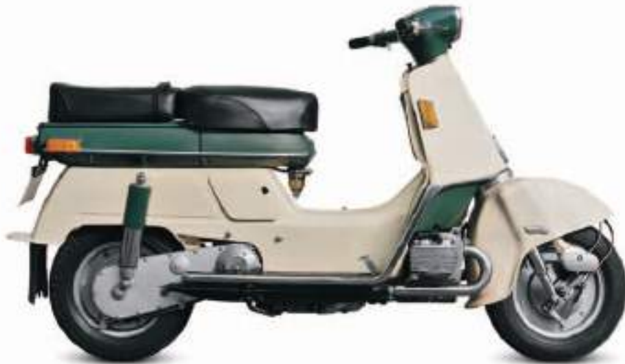
△ Honda Juno M85 1962 Only made for one year the Juno was an innovative steel monocoque scooter with an exposed flat-twin engine and variable hydraulic mechanical transmission. Origin Japan Engine 169 cc, flat-twin Top speed 62 mph (100 km/h)
