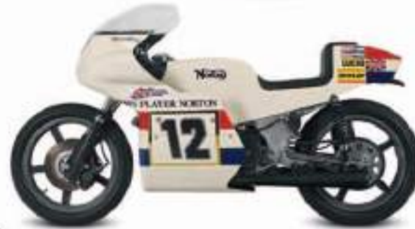
△ Norton F750 1973 Origin UK Engine 746 cc, in-line two Top speed 155 mph (259 km/h)
