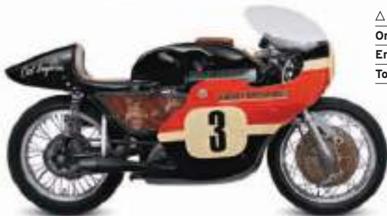
△ Harley-Davidson XR750 1972 Origin USA Engine 750 cc, V-twin Top speed 145 mph (233 km/h)
