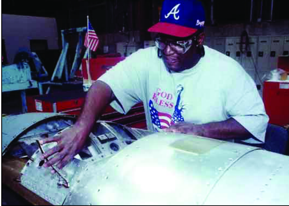
A sheet metal mechanic works on a C-130 oil cooler duct at Warner Robins Air Logistics Center.
