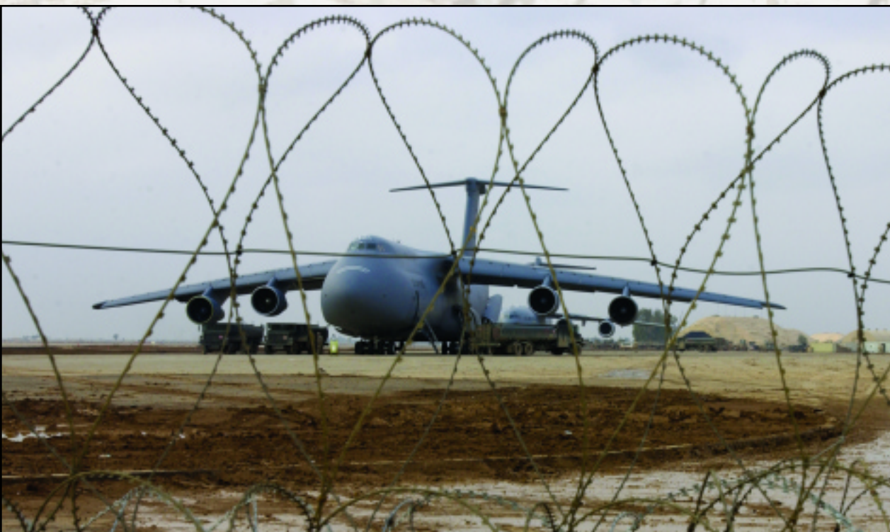
A C-5 Galaxy transport sits on the ramp at Balad Air Base in Iraq. The airfield was certified to receive the C-5 and the 270,000 pounds of cargo it carries. Use of the airfield reduces dependence on ground vehicle convoys to transport supplies.
