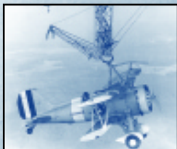
The concept of using a heavy-lift blimp to launch smaller UAVs has a historical basis. In 1933, the Navy used dirigibles as airborne aircraft carriers. Below, the USS Macon retrieves two Curtiss F9C-2 airplanes. Left, a Curtiss F9C-2 Sparrowhawk attaches to the trapeze of the USS Macon.
