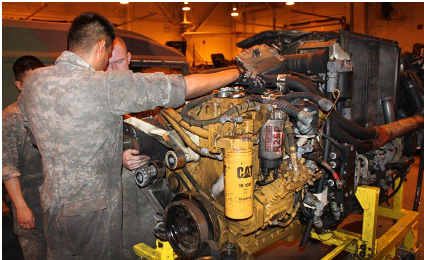
Pfc. Jeremiah Balete, Spc. Xavier Loretto, and Pfc. Gregory Bettencourt, 25th Brigade Support Battalion, 1st Stryker Brigade Combat Team, 25th Infantry Division, at Fort Wainwright, Alaska, repair full up power packs instead of replacing them, saving the unit more than $200,000 on each pack repaired. (Photos by Maj. Karl Beier)
