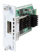
The 3Com Switch 4200G 1-Port 10-Gigabit Module (XFP) 3C17666 shown above adds one XFP-based 10-Gigabit port to the rear of a Switch 4200G system as a high-bandwidth link for connections to high speed network backbones or other peer switches or servers. An XFP transceiver, sold separately, is required to support the desired connection's fiber media.
