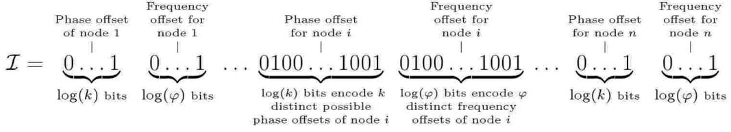
Figure 2.15: Binary representation of search points as a concatenation of grey encoded phase and frequency offsets
