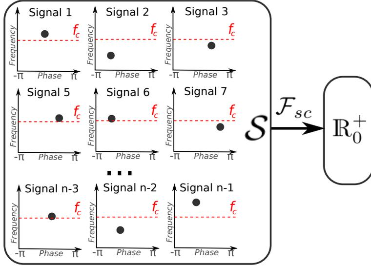
Figure 2.13: Search space and score function for binary feedback-based distributed adaptive carrier synchronisation
