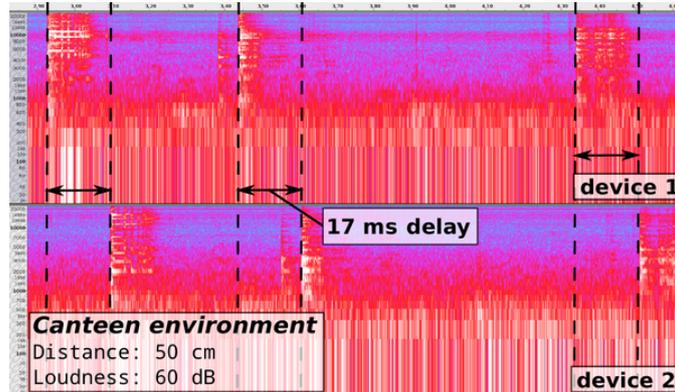
Figure 2.35: Synchronisation offset of NTP synchronised audio recordings (1536-1233/13/\$31.00
