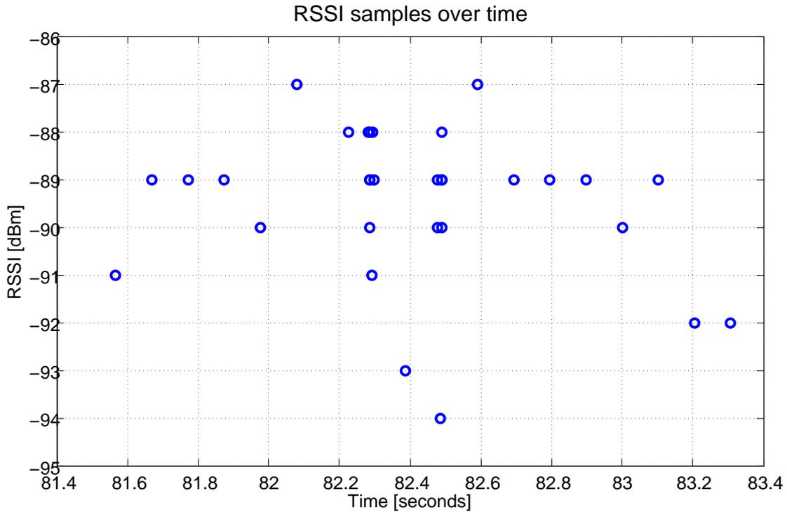
Figure 2.29: RSSI from packets of a single AP (978-1-4799-3445-4/14/\$31.00 ©2014 IEEE)
