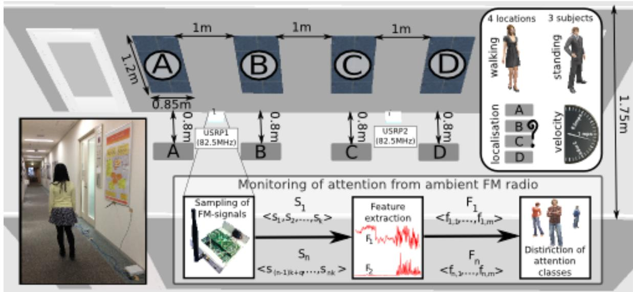
Figure 2.25: Sketch of the evaluation setting. The attention-monitoring system extracted features combining the data acquired by both USRP devices. (Published by the IEEE CS n 1536-1268/14/\$31.00 ©2014 IEEE)
