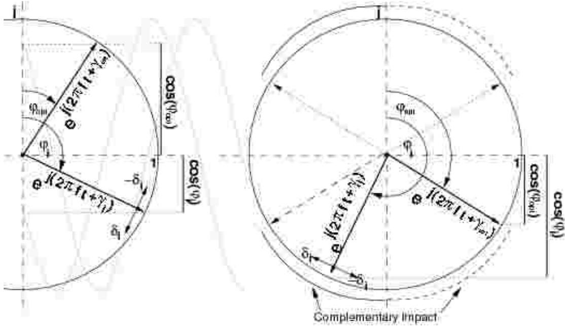
Figure 2.12: Fitness calculation of signal components. The feedback of the superimposed sum signal is impacted by the relative phase offset of an optimally aligned signal and a carrier signal  $i$ . (©2011 IEEE Published by the IEEE CS, CASS, ComSoc, IES, SPS)
