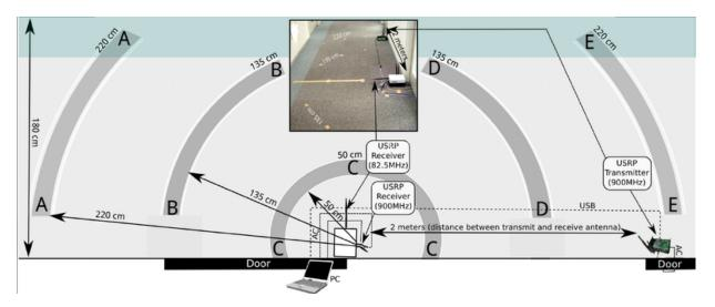
Figure 2.22: Schematic illustration of the corridor in which the case-study was performed. Locations at which activities were conducted are marked (A,B,C,D,E). Both receive nodes are located in the center of the recognition area on top of each other. (1536–1233 ©2013 IEEE)
