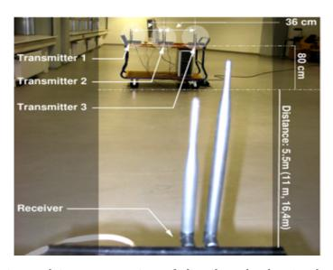
Figure 2.10: Experimental instrumentation of distributed adaptive beamforming among three transmit USRP devices and one receive USRP device. (©2011 IEEE Published by the IEEE CS, CASS, ComSoc, IES, SPS)
