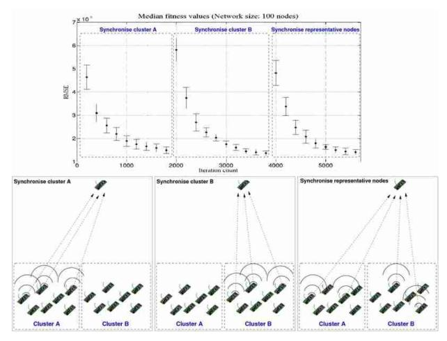
Figure 2.2: Illustration of the approach to cluster the network of nodes in order to improve the synchronisation time of feedback based closed-loop distributed adaptive beamforming. (©2011 IEEE Published by the IEEE CS, CASS, ComSoc, IES, SPS)
