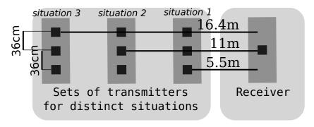
Figure 2.18: Illustration of the experimental setting utilised. Devices are placed on tables with a height of 72 cm.
