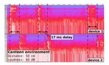
Figure 2.35: Synchronisation offset of NTP synchronised audio recordings (1536-1233/13/\$31.00 ©2013 IEEE Published by the IEEE CS, CASS, ComSoc, IES, SPS)
