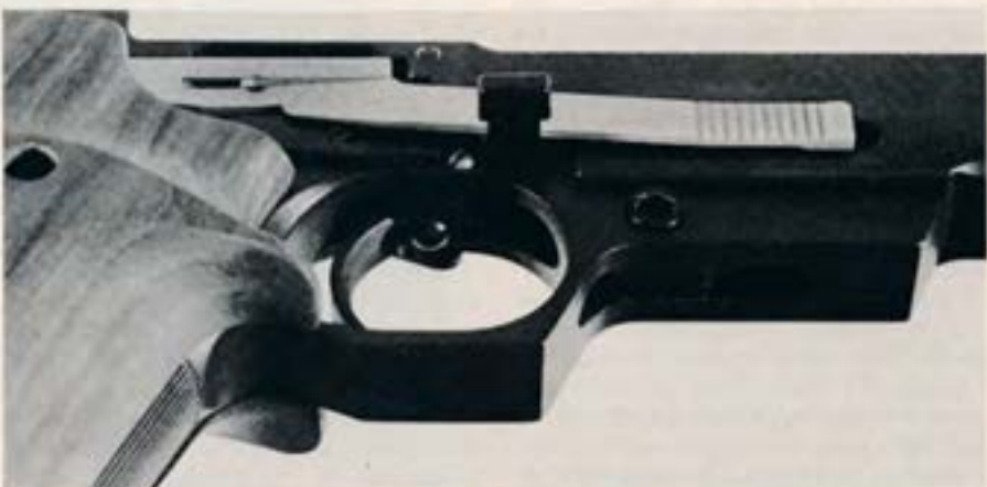
The trigger on the Triace is adjustable for length of pull, over-travel and weight of pull. The allen bolt forward of the trigger holds the unit in place.
