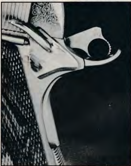
Beavertail grip safety is one of the first ergonomic touches to add.
