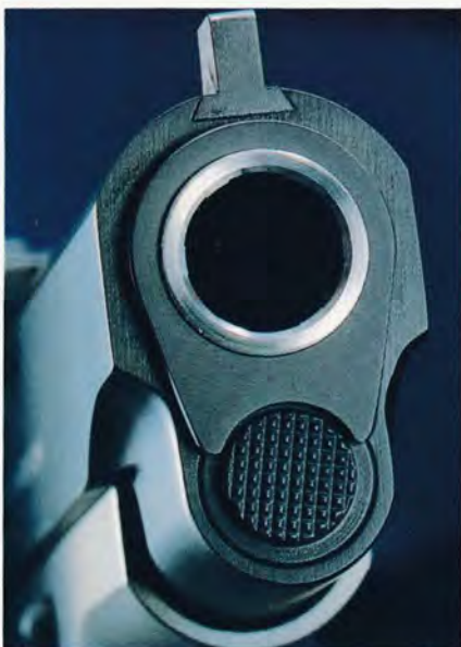
Collet barrel bushing is replaced with solid bushing (above) and front sight with tritium night-sight insert is dovetailed into the slide. The "wings" on the S&W rear sight (right) lend rugged durability to the tritium-inserted adjustable blade. Note the precise checkering on the rear of the slide.
