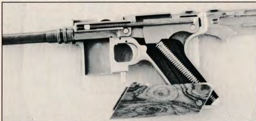
The frame is hinged at the rear, opening like a "clamshell." The toggle lock moves down into the grip. The barrel is instantly replaceable.
