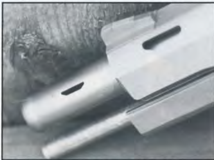
Trapezoidal ports are cut into both barrel and slide to vent powder gas.
