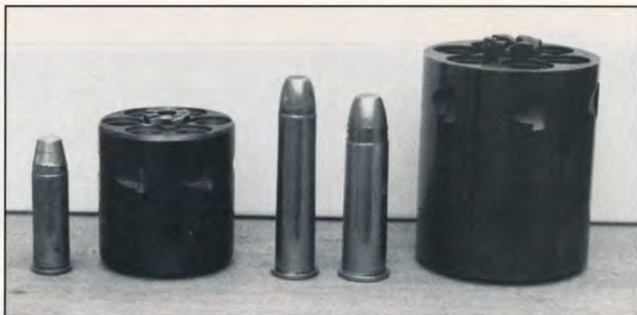
The .45-70 and .50-70 Government cartridges and cylinder (at right) dwarf Elmer Keith's .44 Magnum. The .50-70 can make 1800 fps with the 450 grain bullet.
