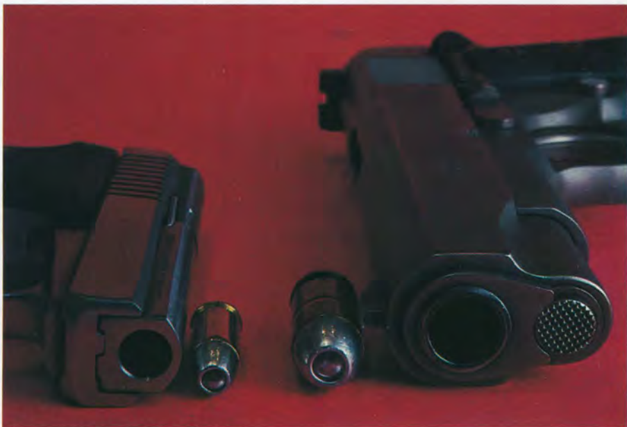
Next to a Colt .45 ACP, the little Seecamp .32 Auto is a pipsqueak. But, as the author points out, the first rule of a gunfight is "Have A Gun," and the Seecamp is a gun! At left, the Seecamp is striker fired, DA-only.
