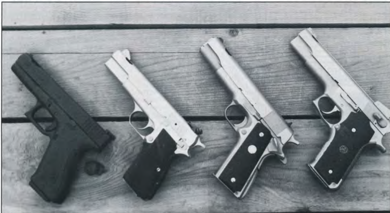
Taffin tested four "autoported" pistols (L to R) a Glock 17 9mm, Browning Hi-Power 9mm, Colt Government Model .45 ACP and a S&W 645 .45 ACP. John said he was impressed with the autoporting process for reducing muzzle rise.
