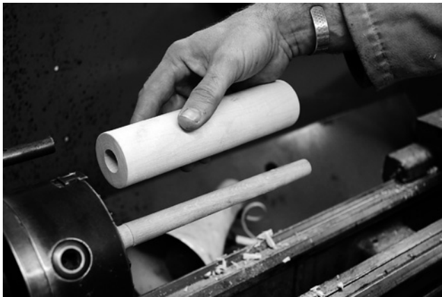
Reaming the bore. Top: Checking the dimensions of the head joint bore. Bottom: The head joint after reaming.
