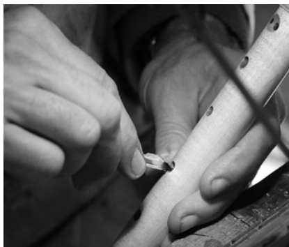
To sharpen a note that is slightly flat, Tim undercuts a finger hole with a scalpel.
