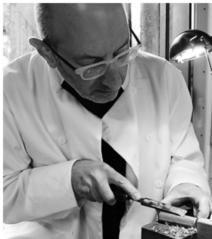
To sharpen a note that is slightly flat, Tim undercuts a finger hole with a scalpel.
