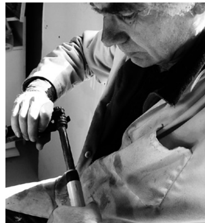
While voicing the instrument, Tim uses a hand reamer to slightly increase the diameter of the bore.
