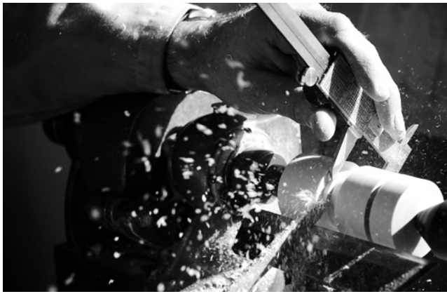
Footjoint and lathe work. Top: Using a lathe to form the exterior contours of the foot joint while checking its dimensions with Vernier calipers. Next: The initial turning of the foot joint exterior, marked with its dimensions and a sketch of its final shape. Last: Finishing the foot joint with superfine sandpaper.
