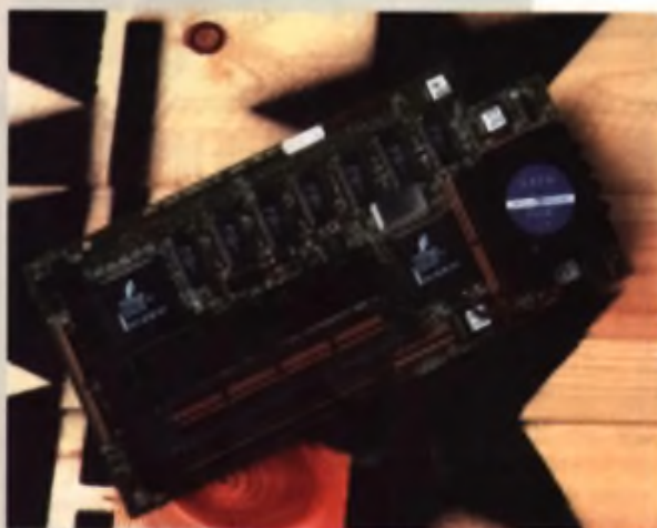
▲ GVP's 4-Faces Accelerator is a Zero card for the A4100 and A3000. As a bonus feature, you get a built-in SCSI connector, allowing additional SCSI devices to be added to your Amiga.
