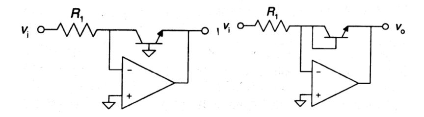
Fig: Transdiode Log Amplifier
