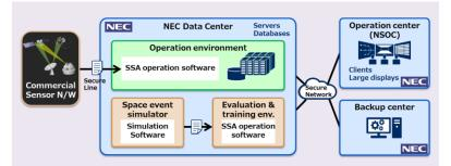
Fig. 2. System configuration of the NEC ComSpOC prototype system
