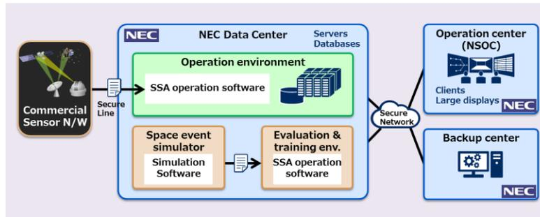
Fig. 2. System configuration of the NEC ComSpOC prototype system
