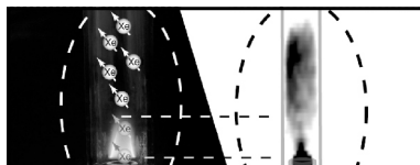
Figure 1.: Sketch showing a photograph of the actual combustion zone (left) and hp ^{129}\text{Xe} MRI (right) of the same region. Dark regions in the MRI indicate high ^{129}\text{Xe} signal intensity.
