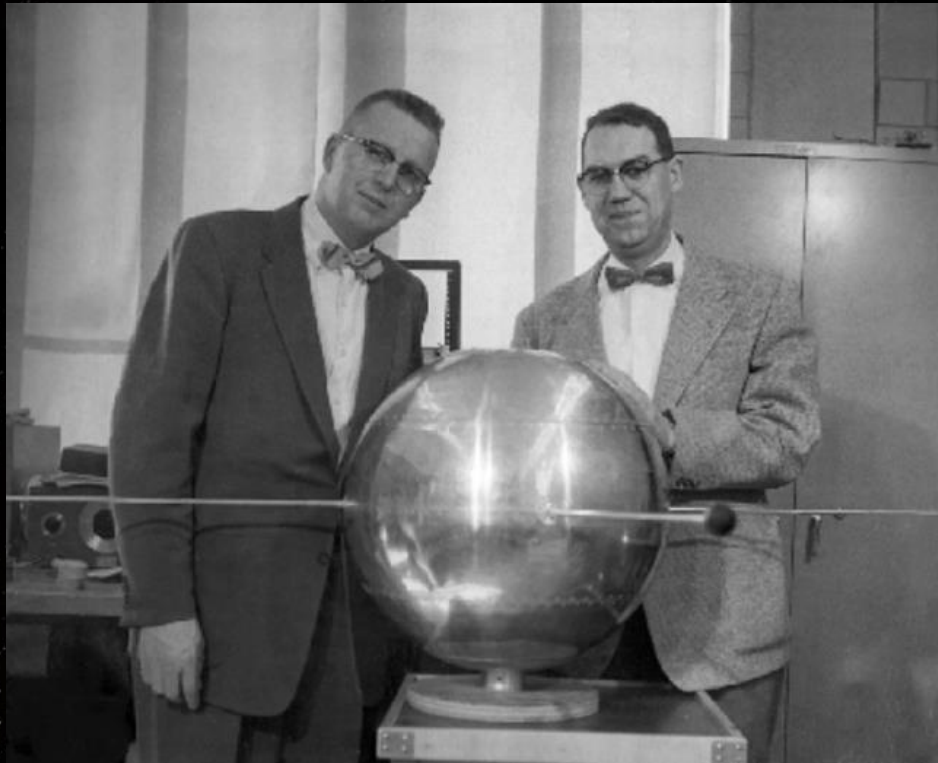
Fig. 1 Professors Suomi and Parent pose with the Vanguard Program's SLV-6 satellite. The Black ball is one of two black and two white spheres as part of their heat budget experiment.
