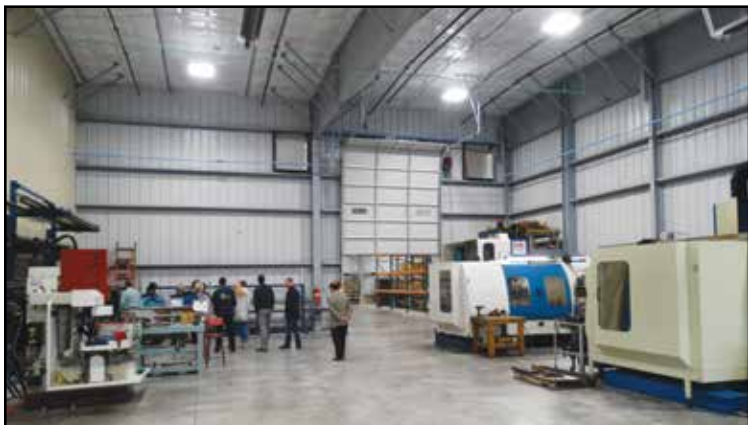
Improvements made in the machine shop where raw materials are prepared for welding include brighter LED lighting and special doors and conveyors leading from the outside directly to equipment for processing. AT/TIM BALDWIN
