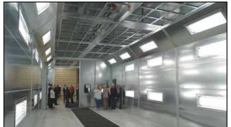
The flow of parts in production moves directly into new painting bays followed by areas that prepare them to be shipped eliminating a need for extensive movement throughout the facility. AT/TIM BALDWIN
