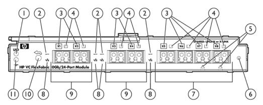
Figure 1 Virtual Connect FlexFabric Module Front Bezel
