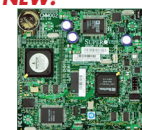
BMB-CMM-002 Mini CMM Installs in SBM-XEM-002M, SBM-IBS-Q3616M and SBM-XEM-X10SM CMM (Chassis Management Module)
