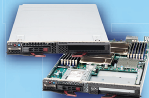
Intel DP Blade w/ PCI-E 2.0 x16 Expansion Slot
