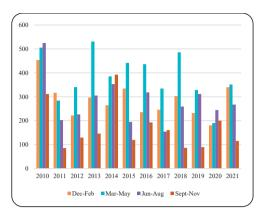
Figure 5. Water level fluctuation at the Brăila station
