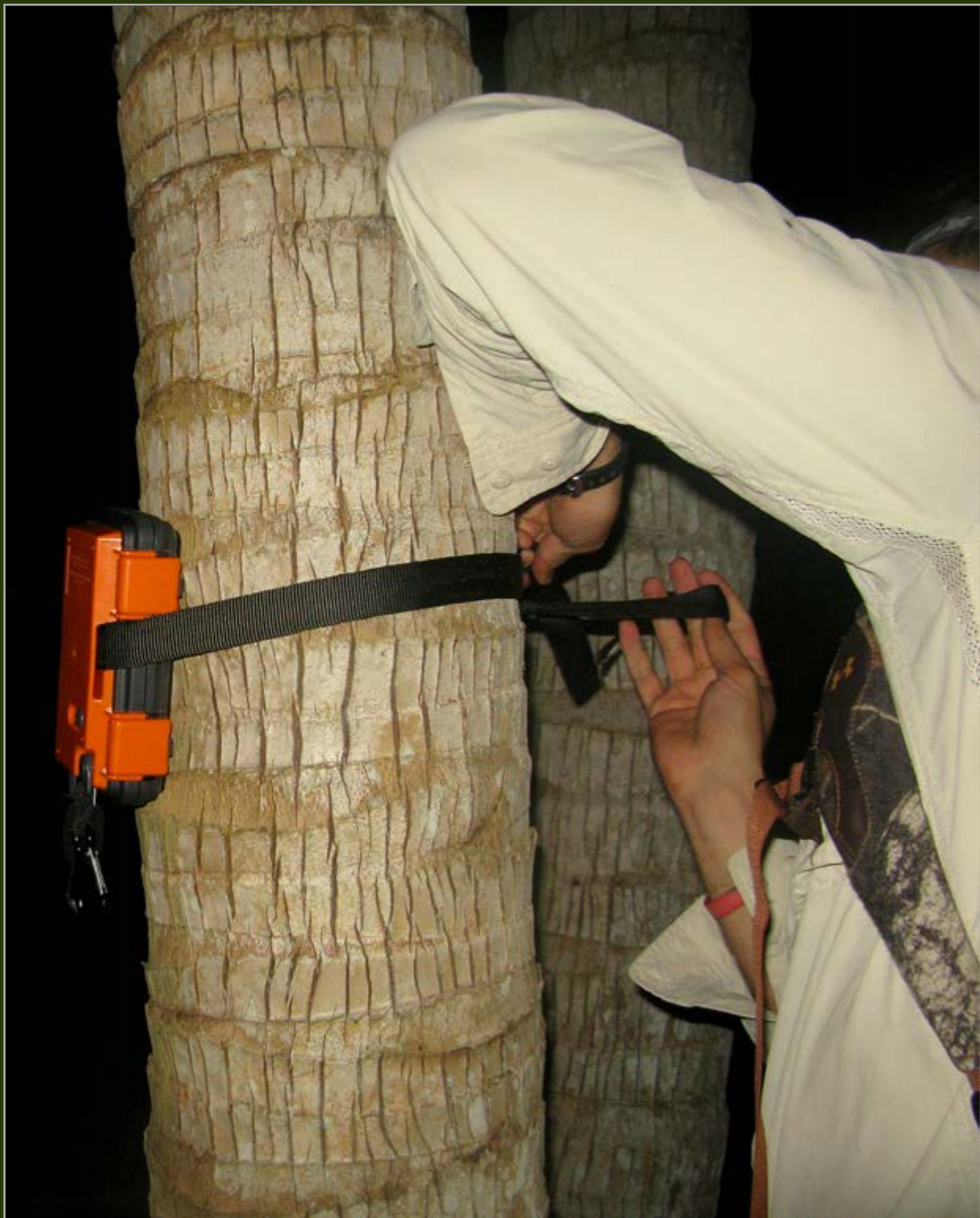
A data logger being placed in situ on a palm tree trunk.
