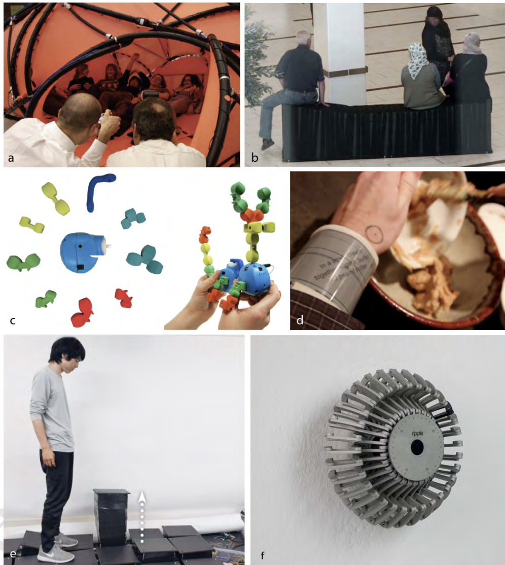
Figure 6.12 A variety of shape changing interfaces and programmable materials, such as, a) The Muscle Body as an example of Pro-active Architecture that is actuated [Oosterhuis and Biloría 2008]; b) coMotion bench to stimulate casual interaction [Kinch et al. 2014b]; c) The Topobo System is a programmable set of toys (courtesy MIT Media Lab); d) DisplaySkin explores the potential of a bendable screen [Burstyn et al. 2015]; e) LiftTiles aim at an adaptable room-scale interior [Suzuki et al. 2020]; f) Ripple thermostat offers expressive and aesthetic interaction [van Oosterhout et al. 2018a]
