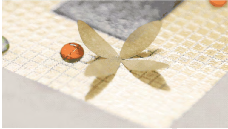
Figure 3.5 Programmable Droplets uses droplets of liquids to change the shape of food [Umaphathi et al. 2018].
