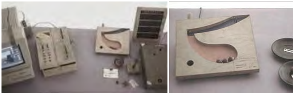
Figure 1.8 Marble answering machine (Durrell Bishop, RCA CRD, 1992): a) System of physical products prototyping object ecologies; b) Closeup of physical marble answering machine prototype. (courtesy Durrell Bishop)
