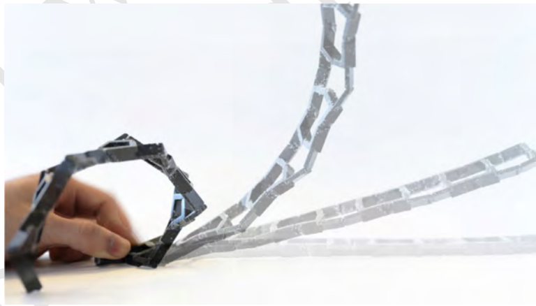
Figure 3.10 A 1D tessellation of spatial transformation of bending and twisting. This tessellation creates a curling strip [Ou et al.].
