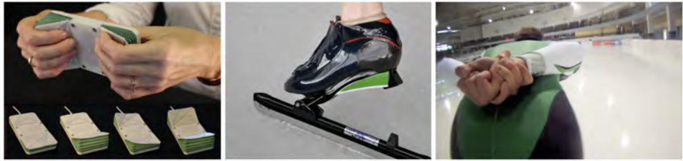
Figure 6.2 The direct or embodied approach towards TEI, e.g. Reflex, a shape-changing phone [Rasmussen et al. 2016], and Augmented Speed-skate Experience, a sonification device to enhance speed skating skills [Stienstra 2016; Stienstra et al. 2011]
