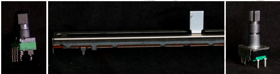
Figure 5.6 rotary potentiometer, linear potentiometer, and rotary shaft encoder
