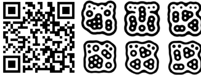
Figure 5.10 Example fiducials for CV recognition: a) QR code [Public Domain 7 ]; b) ReactIVision codes [Kaltenbrunner 2009a]
