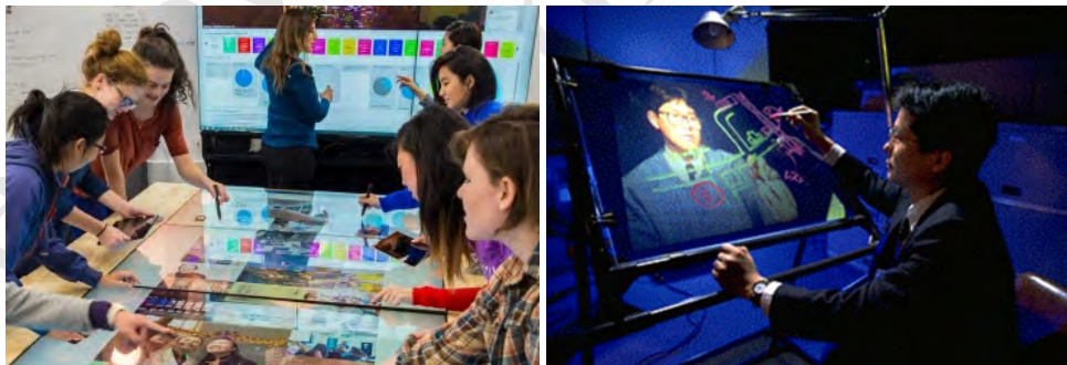
Figure 5.15 Pixelated display variants: a) multitouch and object-sensitive tabletop display (photo courtesy of Orit Shaer); b) ClearBoard: transparent OLED display [Ishii et al. 1994]
