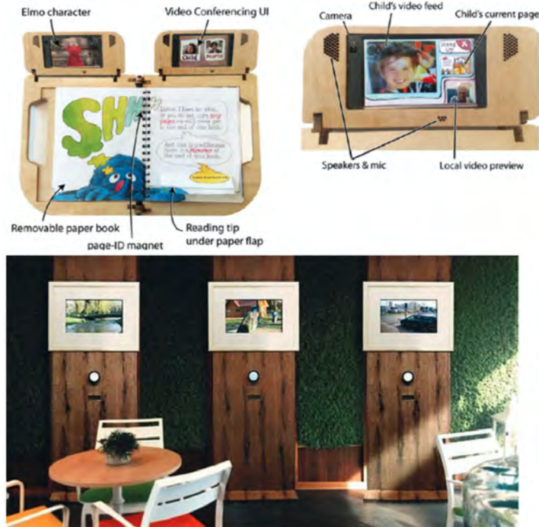
Figure 2.10 TEI approaches for increasing social connectedness and engagement of older adults. Top: Family Story Play [Raffle et al. 2010]; Bottom: ViewBricks [Lin et al. 2016].
