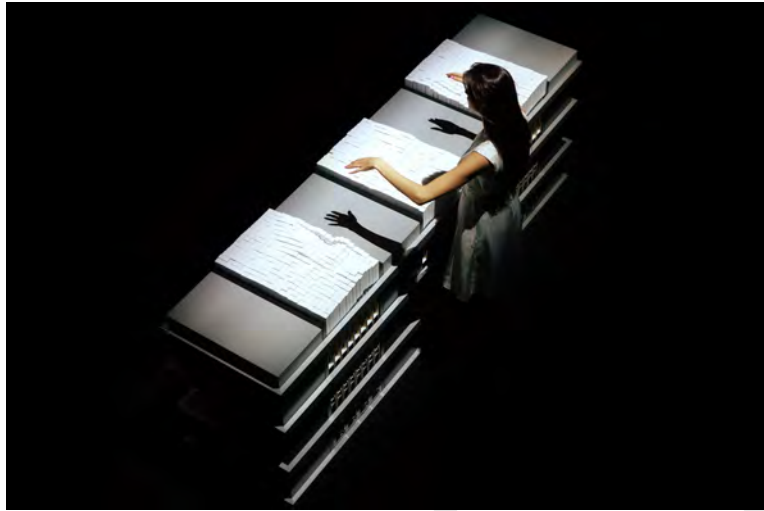
Figure 3.4 Transform – dynamic furniture that senses kinetic energy and transforms it into dynamic movement [Ishii et al. 2015b].
