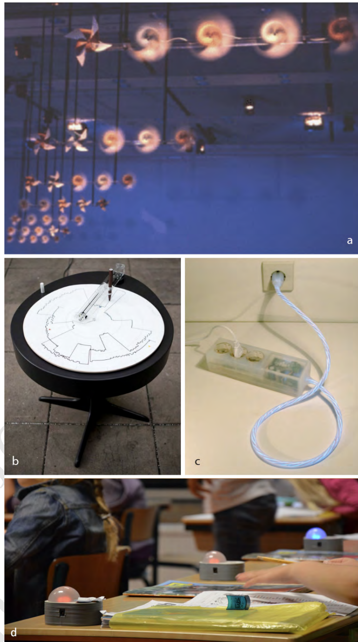
Figure 6.14 Various examples of peripheral perception and interaction, for example, a) Pinwheels, displaying ambient information (courtesy MIT Media Lab); b) Sidetrack, visualizing people's movement patterns [Barcikowski et al. 2010]; c) Power-aware Cord, visualizing energy usage [Gustafsson and Gyllenswärd 2005]; d) FireFlies for communication at primary schools (photo Saskia Bakker).
