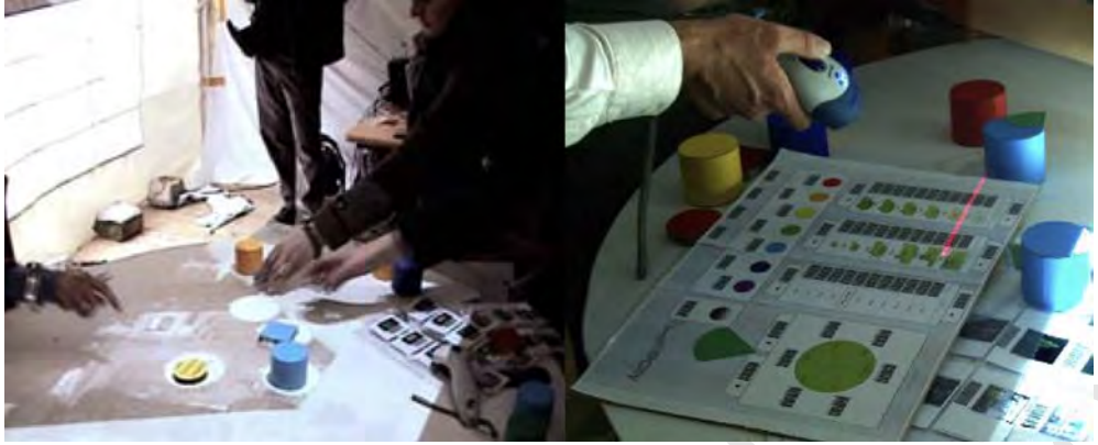
Figure 8.4 ColorTable, a table-based interface that supports co-construction for urban planners and other stakeholders [Maquil et al. 2008]
