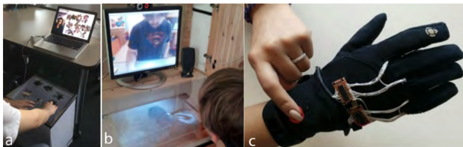
Figure 2.9 a) Puzzle Space allows long distance couples to solve a puzzle together with tangible and digital components (Photo Credit: Rui Pan); b) ShareTable allows for easy videochatting and an interactive tabletop task space to facilitate communication; c) Flex-N-Feel allows for a sense of touch for long distance couples (Photo Credit: Samarth Singal ) [Pan et al. 2017; Singhal et al. 2017; Yarosh et al. 2013].
