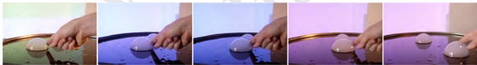
Figure 3.8 The Soap Bubble Interface makes users interact with fragile bubbles to interact with the computer. A user moves a smoke-filled soap bubble in order to influence the room illumination [Sylvester et al. 2010].
