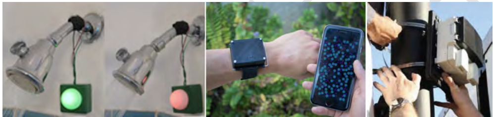
Figure 8.7 Citizen Science encourages broad participation of non-experts in science and engineering. Left: UpStream is a project that uses ambient displays to raise awareness about water consumption and promote conservation in public and private spaces [Kuznetsov and Paulos 2010b]. Middle: MyPart is a wearable, personal particle sensor that allows users to track and visualize air pollution [Tian et al. 2016]. Right: A sensor package mounted onto a street sweeper, transforming it into research vehicle for monitoring air quality and analyzing the environmental action landscape [Aoki et al. 2009].
