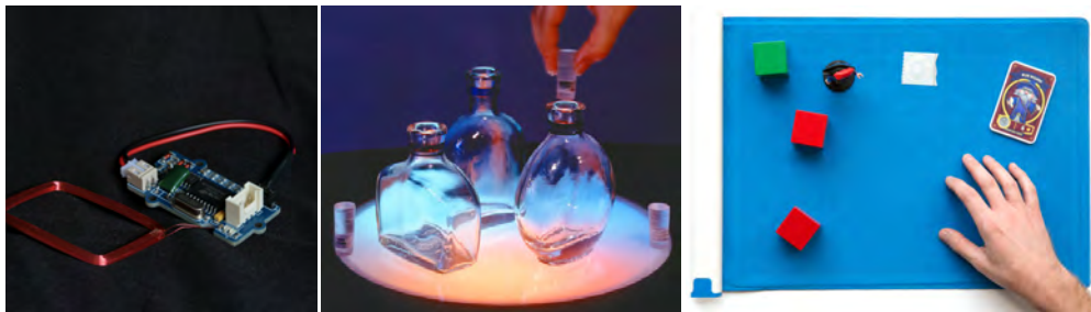
Figure 5.11 RFID/NFC sensors: a) Grove/seed [photo courtesy Brygg Ullmer]; b) music bottles (analog + digital tags); c) Microsoft Zanzibar NFC + multitouch sensing 2D array sensor
