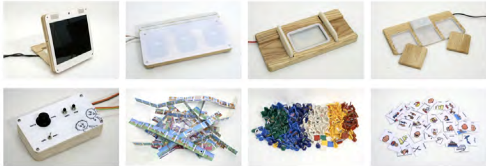
Figure 8.10 The LinguaBytes system, created for developing verbal skills in children. Clockwise from top left: the output module for displaying interactive content, the base module, the story module, the exercise module, cards, input figures, story booklets, and the control module [Hengeveld et al. 2013b].
