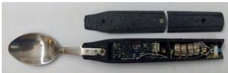
Figure 2.12 DataSpoon monitors movement kinematics during self-feeding for children with motor disorders [Zuckerman et al. 2016].
