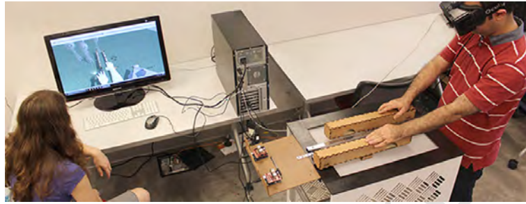
Figure 7.3 User evaluation of the Tangibles for Augmenting Spatial Cognition (TASC) system [Chang et al. 2017a,c]. The system employs tangible and embodied interaction in virtual reality to engage users in a series of spatial puzzles that are designed to support and enhance their perspective taking spatial ability.
