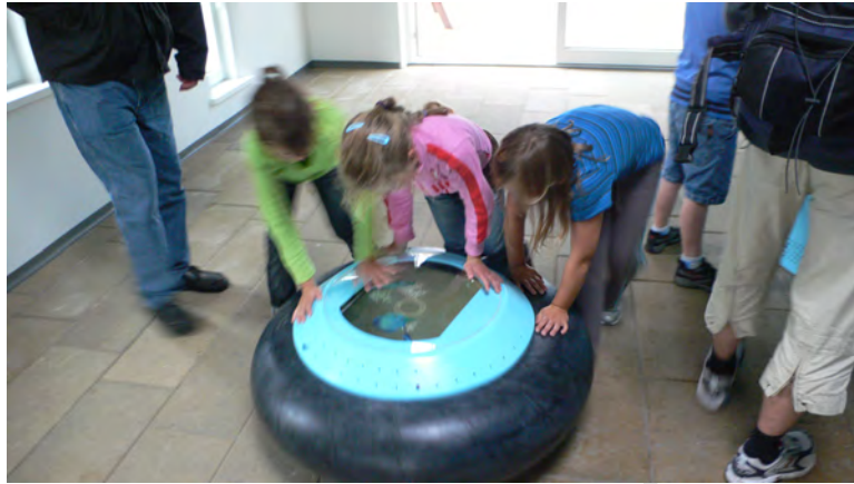
Figure 3.14 Hydroscope: this Peephole experience allows users to look down into the digital ocean through the hydroscope, and encourages active exploration through pushing the hydroscope around the floor to reveal more of the ocean (photo courtesy Christian Dindler). [Dindler et al. 2007]
