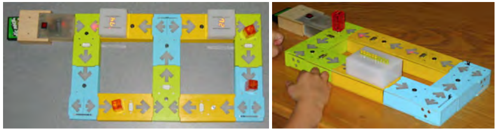
Figure 7.1 FlowBlocks [Zuckerman et al. 2005] is a TUI-based modeling and simulation environment consisting of wooden blocks with embedded computation that are connected to create models of data flow structures.
