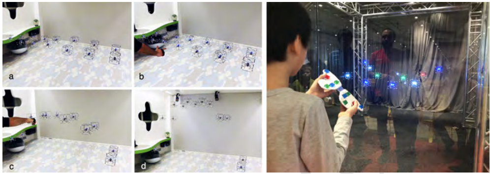
Figure 8.20 Left (a-d): A user creates an archway from a 2x7 grid of GridDrones via ray casting with a "Point" gesture to select keystones. Once the keystones are selected, the user can manipulate them using a phone application. Right: A child interacts with the GridDrone butterfly animation using an embodied controller [Braley et al. 2018b].
