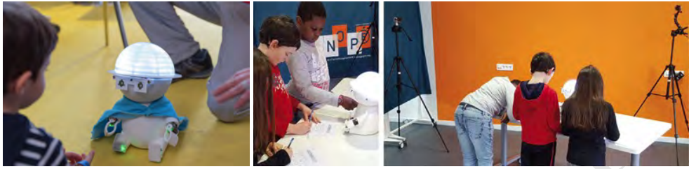
Figure 7.2 Left: Teegi [Fleck et al. 2018] is a physical puppet that lights up to display areas of brain activity as children interact with its limbs and eyes. Middle/Right: children interact with Teegi during a user study that took place as part of a science workshop [Fleck et al. 2018].
