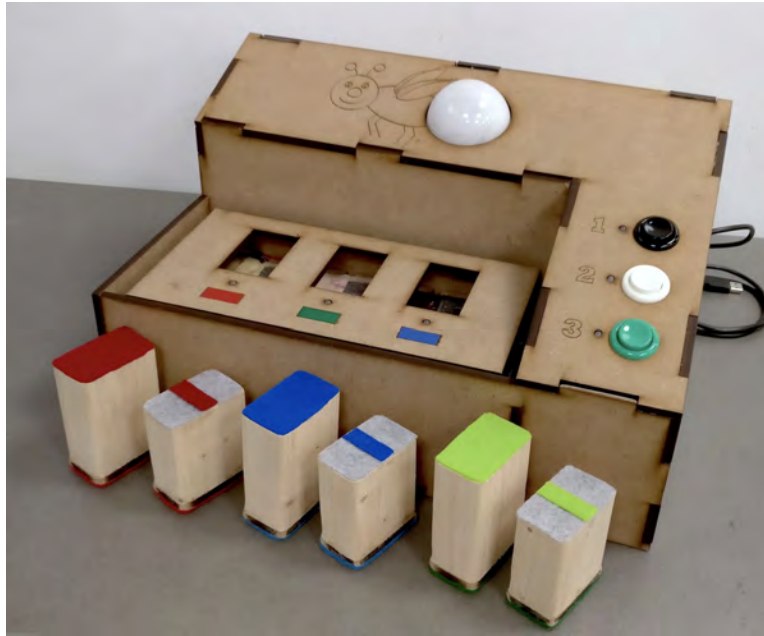
Figure 2.6 The current prototype of CRISPEE. Tangible blocks code red, green, and blue light to be either on (solid color) or off (colored line). Blocks are placed into the corresponding slots on the platform to create the genetic program of the firefly, with a colored output in the firefly's tail [Verish et al. 2018].
