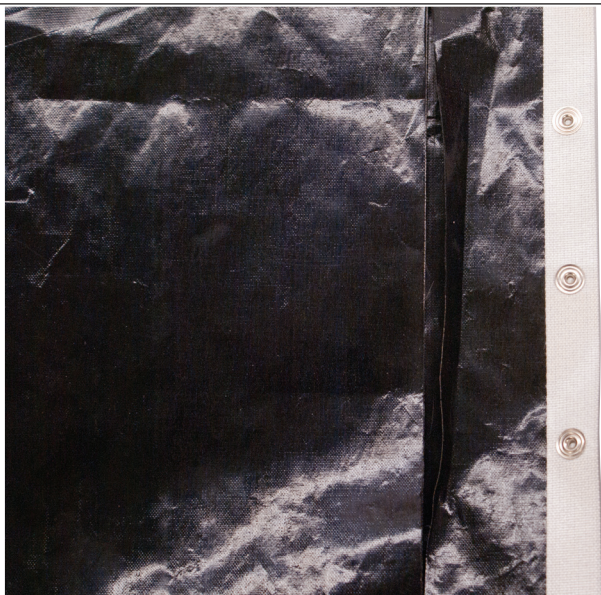
BELT IS TORN AND FOLDED. REPLACE BELT.
