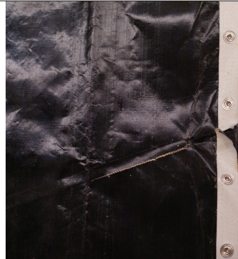
BELT IS MISSING SNAPS AND IS DAMAGED. REPLACE BELT.
