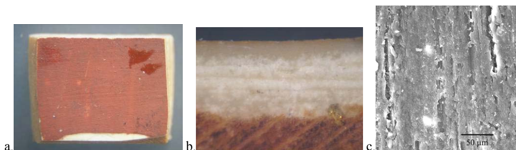
Fig. 18 - Deposits and infiltrations of residual substances on the painted wood after the permethrin treatment in shellsol D70: macroscopically (a), stratigraphy under the stereo magnifying glass (b) and SEM (c)
