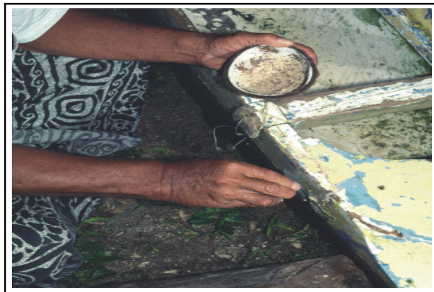
Samoa 3. Canoe caulking using paste from Atuna racemosa fruit.
