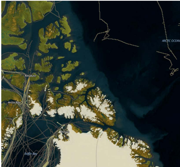
Figure 34. Ship traffic density in the LIA region illustrated by a scale from yellow (low traffic) to red (high traffic). Ship traffic density indicates the intensity of shipping as a function of the size and number of ship tracks in a 5 x 5 km grid. The ship traffic observations are made through the satellite based Automatic Identification System (AIS), which provides the identification of the spatial location of a vessel at a given time. Automatic System AIS data are provided by The Norwegian Coastal Administration www.havbase.no 2012 and further processed by DNV and WWF. Map made by arkgis ( www.arkgis.org ).
