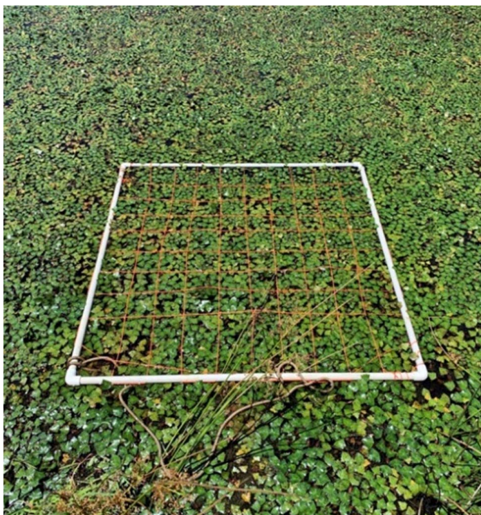
Figure 4. Quadrat used for sampling T. bispinosa coverage (QC). Whole quadrat is 1 m by 1 m and is divided into 100 squares each 0.1 m by 0.1 m.
