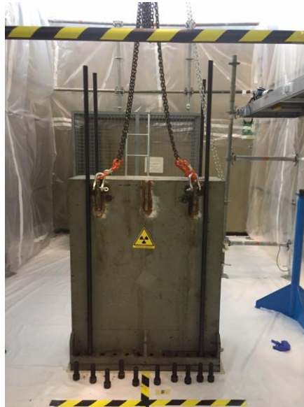
Figure 1 – HEU converter inside the steel shielding
