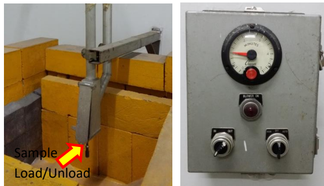
FIG.2. Pneumatic transfer system: (a) Sample load/unload unit, (b) controller
