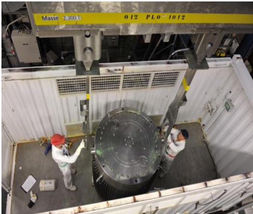
Fig. 3 and 4: TN ® MTR cask loaded in a 20 feet ISO container for transport
