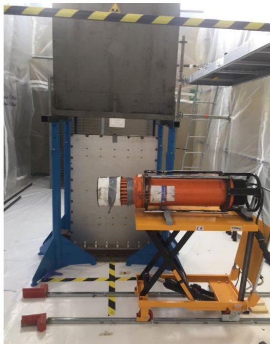
Figure 2 - The X-rays equipment and the positioning of the system
