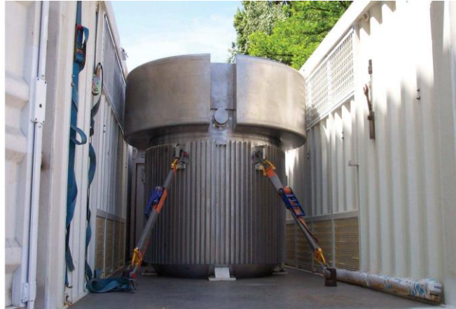
Fig. 3 and 4: TN ® MTR cask loaded in a 20 feet ISO container for transport
