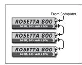
In the leftmost column, a set of interfaces is depicted in the required order; DigiLink connections are shown as well.
