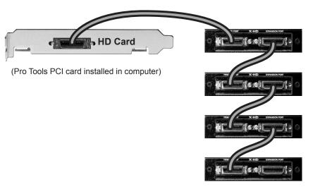
(X-HD Cards installed in Apogee converters)
