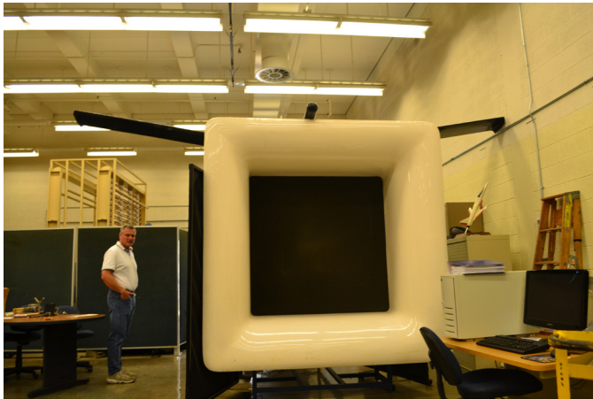
Picture of the front of the wind tunnel where the air is sucked in.
