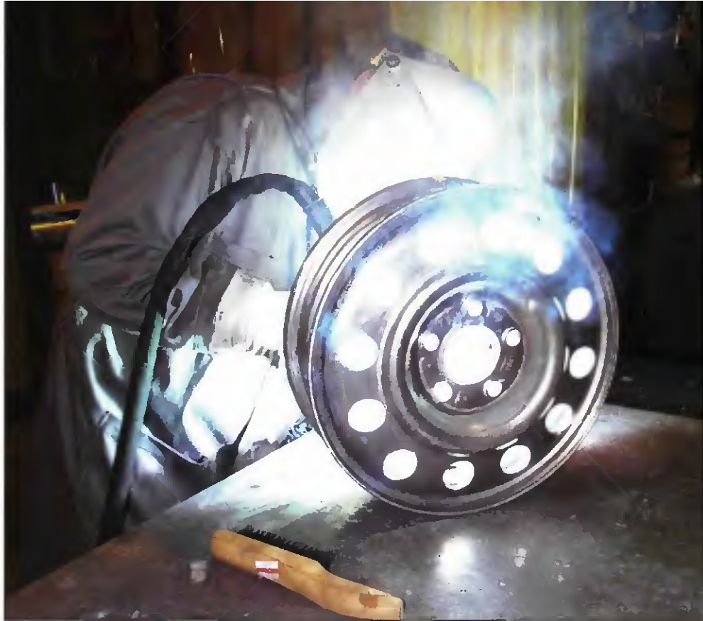
These days, almost all aluminum welding is performed using GMAW or GTAW. With those two processes, flux entrapment, which could lead to corrosion problems, is not an issue.
