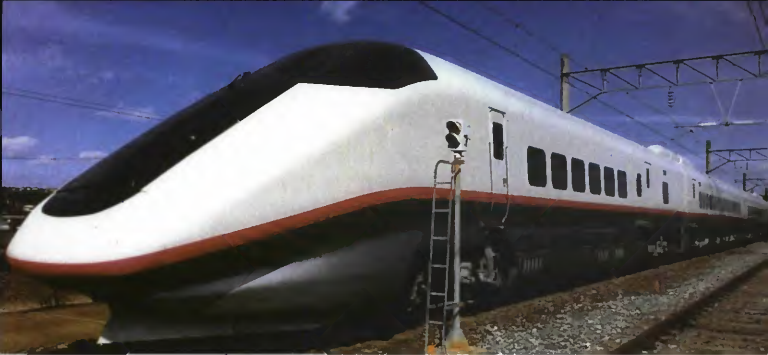
Fig. 2 — Type E3 trains attain speeds as high as 170 mi/h.
