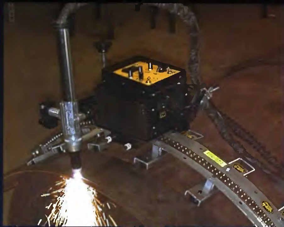
MODULAR WELDING TRAVEL CARRIAGE Runs on three different rail systems. Mix and match components.
