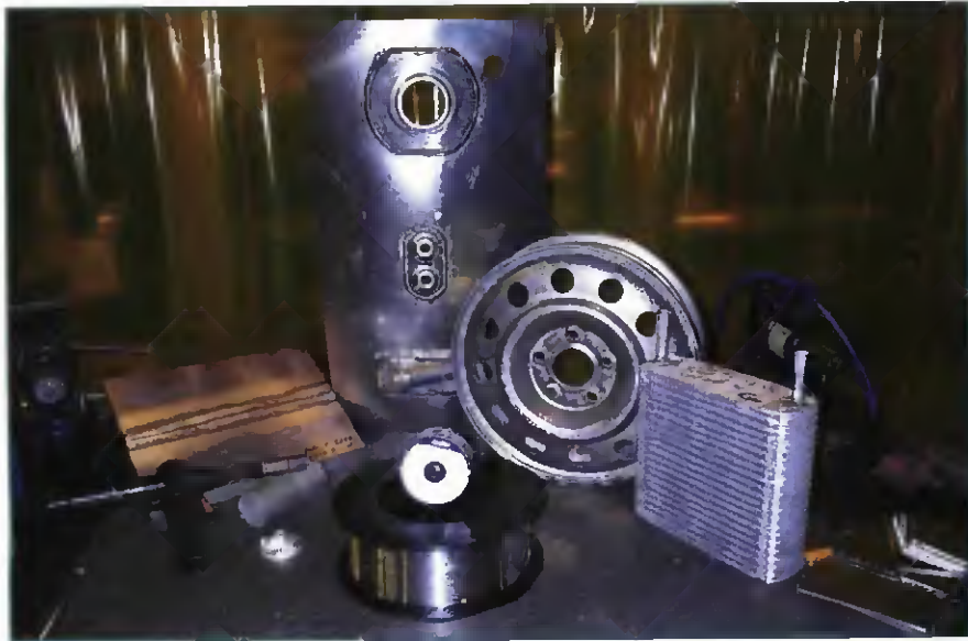
Fig. 1 — Various welded structural aluminum parts. Unlike steel, where the filler metal is usually matched with the tensile strength of the base metal, many aluminum alloys can be welded with any one of a number of filler metals.
