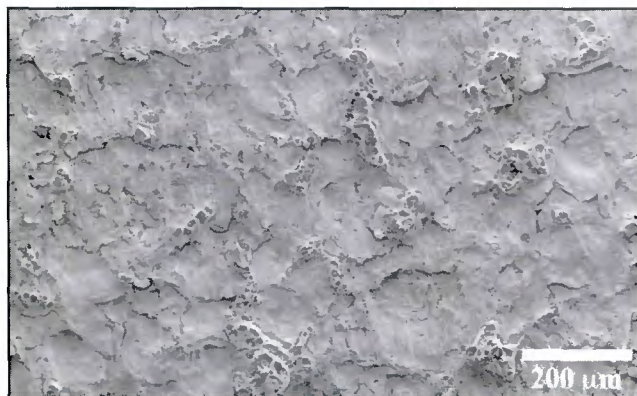
Fig. 1 — SEM micrographs of the fracture surface on one of the edge-detonated Izod samples.
