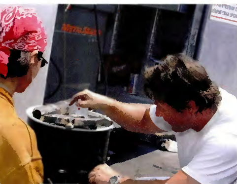
Floyd Elliff of Local 263 (on right) tests the weld coupon of April Finkbonner from Local 86. This weld shows a slightly convex appearance, so it passes this portion of the weld test.
