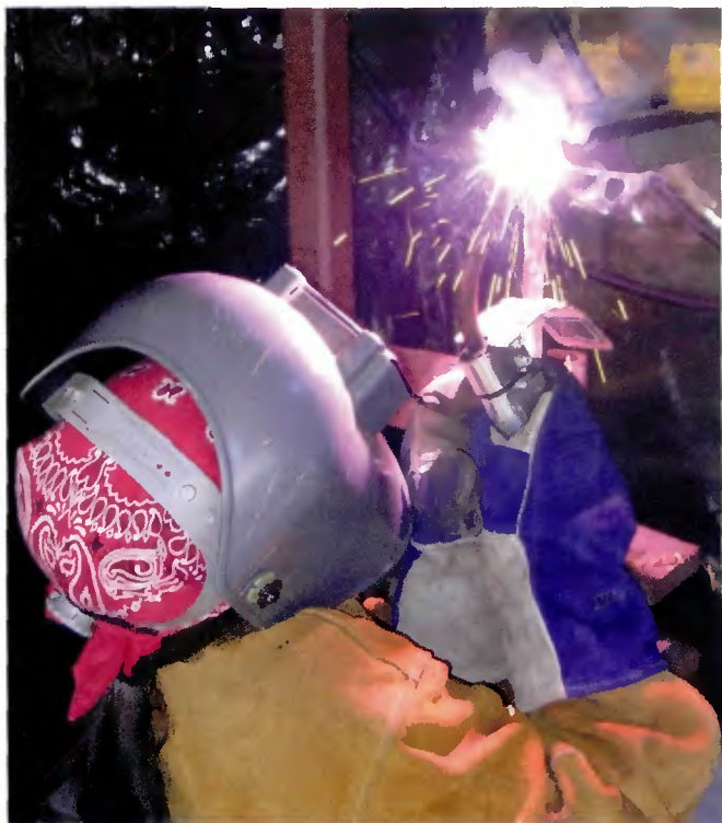
Fig. 1 — For good results when welding with AWS E71T-8 flux cored wires, maintain a proper electrode extension ( \frac{1}{4} in.) and use the proper gun angle (5 to 10 deg toward the direction of travel).
