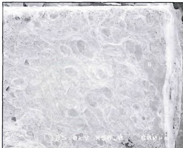
Fig. 14 — Fractography of a porosity-containing, fatigue-tested specimen.
