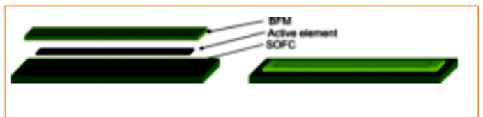
Fig. 2 — Schematic diagram of the PVD-layer composition.
