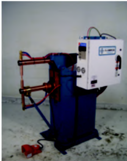
Fig. 1 — A 50-kVA rocker arm spot welding machine. A machine like this, manufactured to RWMA standards, is a good general-purpose machine. The modern control improves welding quality, and a built-in SOFT-TOUCH system protects the operator from pinch-point injury. A reputable dealer who asks lots of questions about how the machine will be used can be a great help in explaining the many machine and control options available today.
