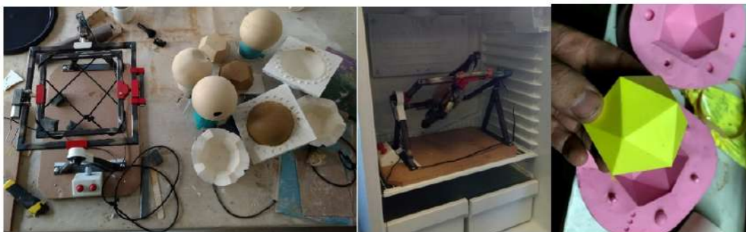
Figure 12: Machine testing with rotocasting ceramic, chocolate & thermosetting resins.
