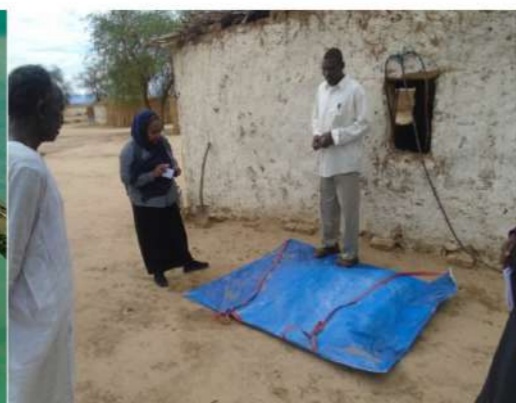
Figure 4 Biogas storage bag in use outside the kitchen (Farah, 2018).
