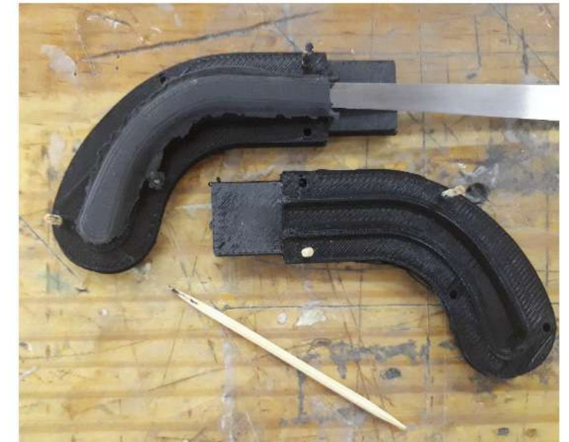
Figure 6: 3D printed moulds were used to mould air-drying clay around temple tips
