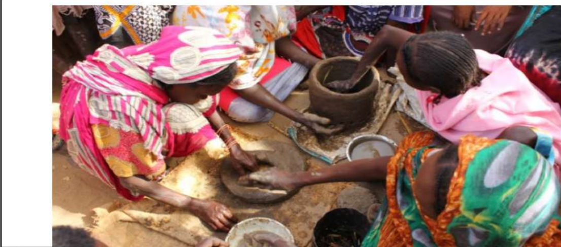
Figure 9 Women's pottery workshop: women produced gasifiers then tested the stove with solid waste derived fuel and produced biochar.
