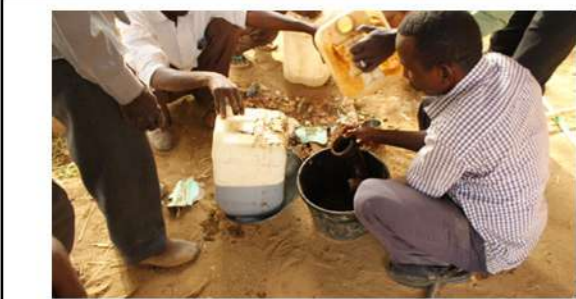
Figure 7 Biogas experiment in Kass vocational school: 16 litres jerry-can filled with crushed goat manure
