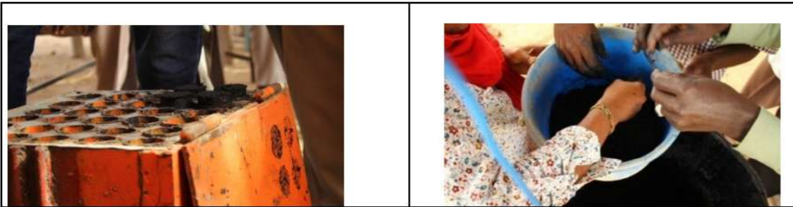
Figure 6 Gasification experiment in Kass vocational school to produce briquettes; The materials and tools applied use a locally available binder (okra powder) compacted by the use of a mechanical press
