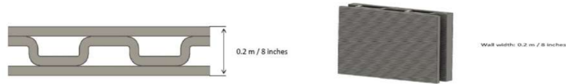
Figure 12: Wall design using Apis Cor 3DCP (Apis-cor, 2019)
