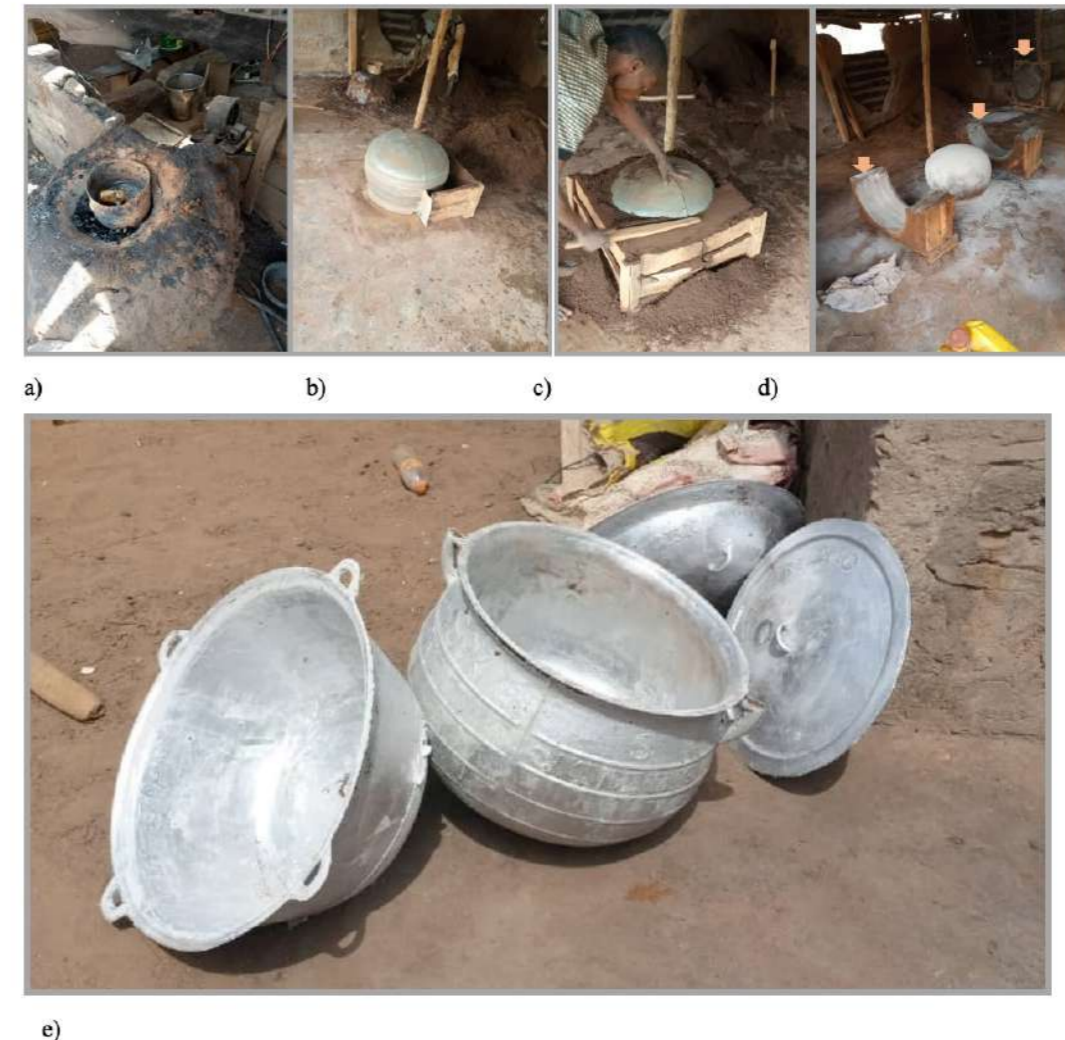
Figure 3: The making process and final products of artisanal aluminium sand-casting technique, Saki, Nigeria: a) melting of aluminium scraps in a furnace; b) a sand-filled pot pattern set with a wooden modular flask (drag); c) a two-part split drag packed with sand; d) a sand core with the flask mould separated (arrows pointed at the cope and the split drag); e) final aluminium cast products (pots) waiting to be fettled. Photographs taken for the authors by Jesutoba Gbadegesin (2020), used with permission.
