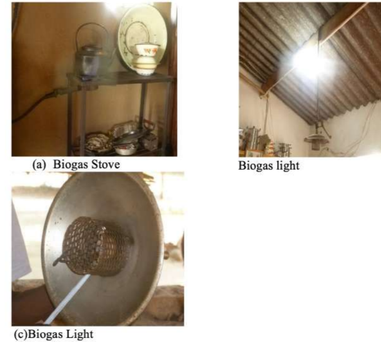
Figure 6: Biogas use (a) Biogas stove (b) Biogas light and (c) Biogas light
