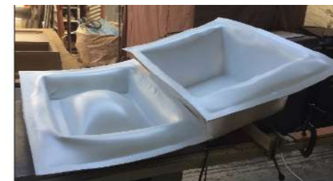
Figure 11: Failed attempts at making large mould parts in South Africa (Brown, 2017).
