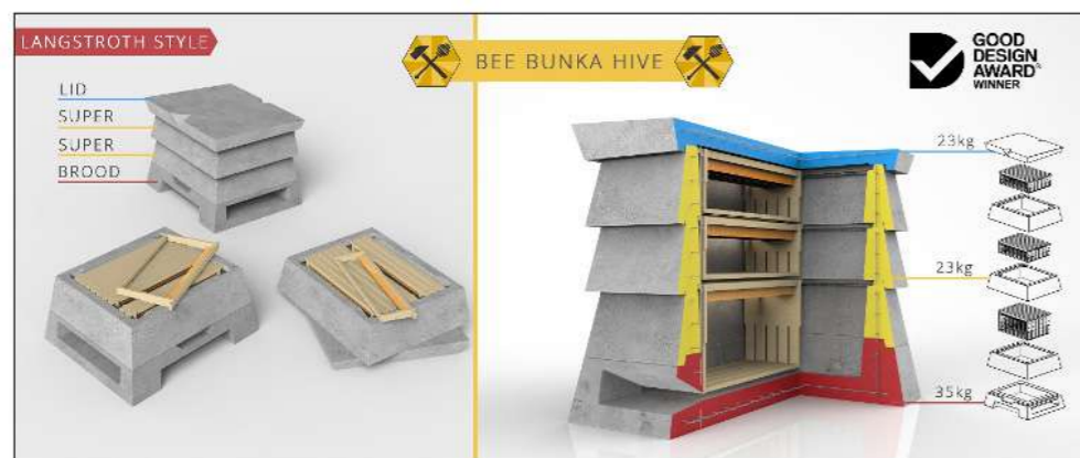
Figure 6: The Beegin Bee Bunka - lightweight concrete beehive, (Brown, 2018).
