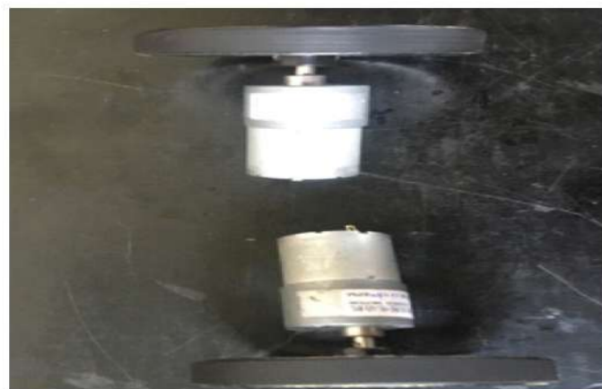
Figure 3: DC motors connected to the tires
