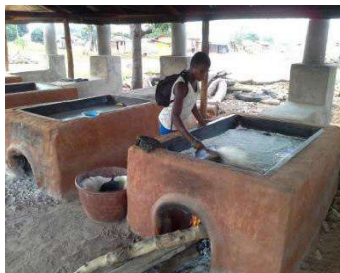
Picture 2: The retrofitted stove in use.
