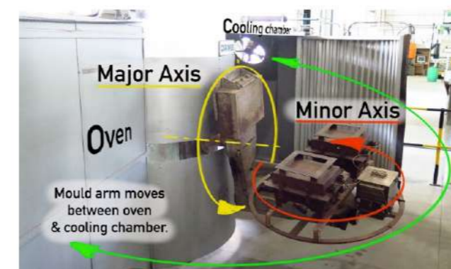
Figure 1: Industrial rotational moulding machine (image by author).
