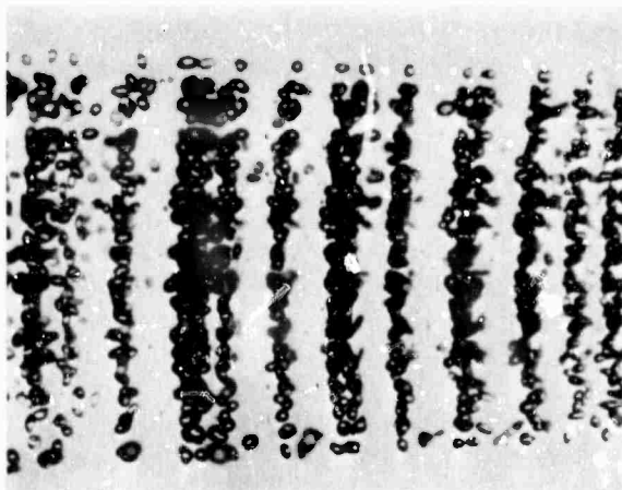
Figure 11.26.--Water spray produced through a perforated-plate nozzle having 0.008 in. diameter holes at 5 p.s.i., 8 in. from the nozzle. (A) Still air, (B) 75 m.p.h. airstream (3.5X).
