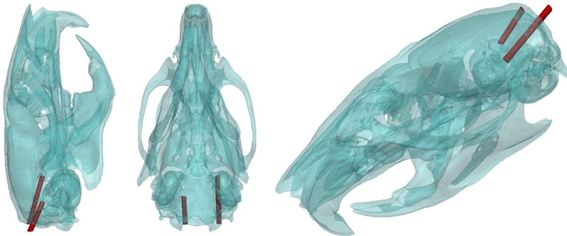
Figure 15 A depiction of the sensor location within test specimen 2 with a cranial, lateral, and isometric view. The skull is shown in blue and the cannulas are shown in red. This specimen was used in Task 2.
