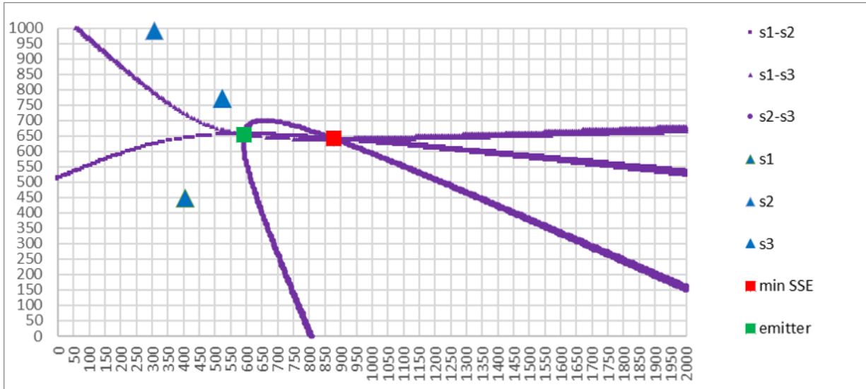
Figure 22: Three immersed sensors at nominal altitudes of 100 m, without position or timing errors, where the point that has the minimum SSE is 286 m from the true position of the emitter. Parameters: N = 3 immersed sensors, side = 1,000 m, alt = 100 m, error-free.
