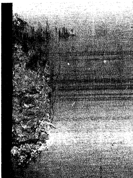
FIGURE 7 Macrograph of the galled region and vertical wear marks on the outer diameter of the pin. Mag. 12.5x.
