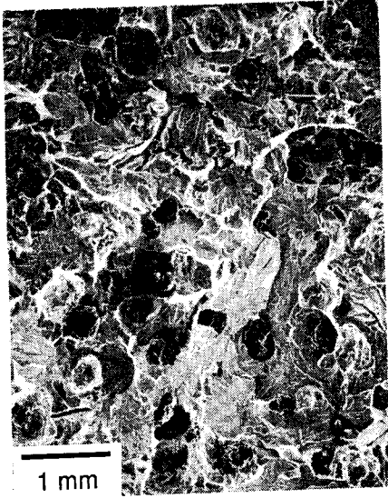
Figure 11. SEM fractograph of the ductile iron tensile specimen showing minor secondary cracks in the matrix.
