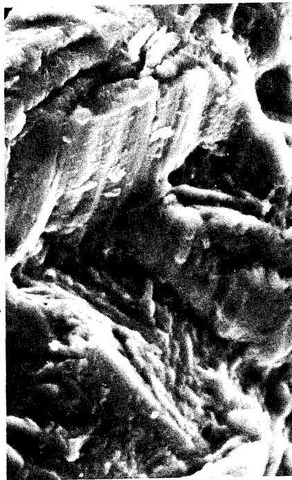
FIGURE 28 Fractograph depicting the characteristic fatigue fracture surface observed on the ARL-MD bend beam specimens. Mag. 1,000x.
