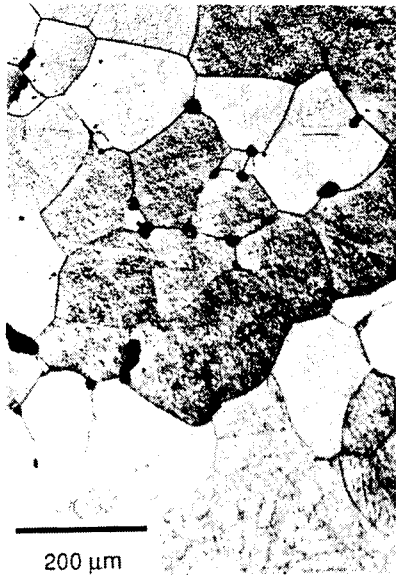
Figure 3. Equiaxed microstructure of a heat-treated 771.0 Al sample showing both angular and spherical cavities and secondary constituents.
