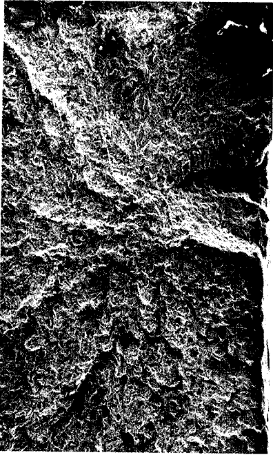
FIGURE 17 SEM fractograph showing the fracture origin and radial marks. Mag. 50x.
