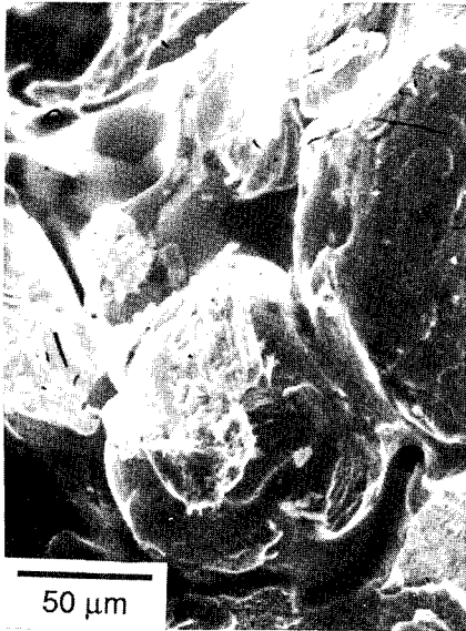
Figure 7. Sickle-shaped intergranular cavities in the Al trunnion casting.
