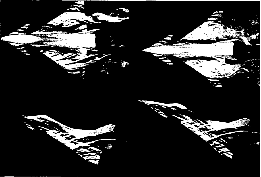
Water tunnel flow visualization illustrates the vortex flow structure over the wing of a highly swept canard-wing-body fighter configuration at two angles of attack. (From MBB)
