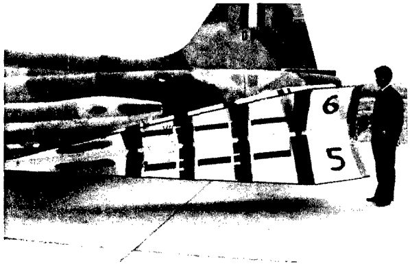
The Flight Mechanics Panel sponsored a project to help Greece develop a capability in store separation techniques. Although intended mainly for bombs and pods, it was also used for a Dart towed target, as shown here.
