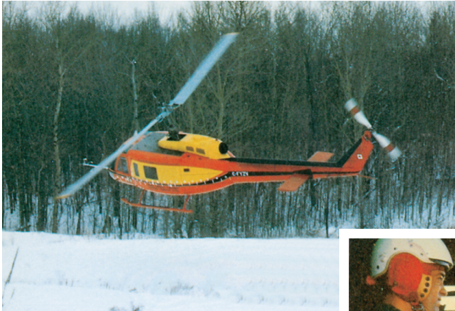
This helicopter belonging to the national aerospace establishment of Canada was configured as an airborne simulator to evaluate control strategies, pilot interfaces and handling qualities for helicopters, particularly in "nap of the earth" (NOE) operations.
