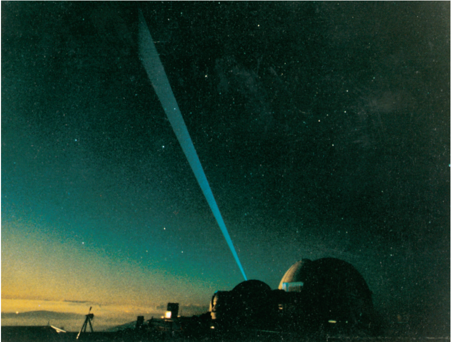
Time-lapsed photograph of a laser beam during an atmospheric experiment to correct for phase distortions introduced by the atmosphere.
