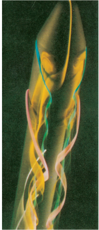
Model of conceptual European fighter undergoing tests in the German/Dutch (DNW) wind tunnel.
