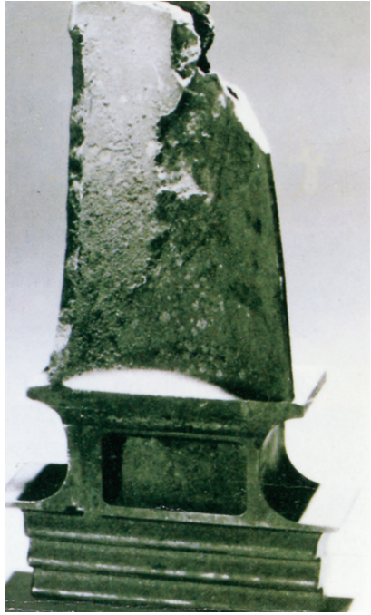
Hot corrosion of gas turbine blade.
