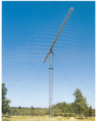
A Horizontal Log Periodic Antenna used for high frequency communications research in difficult propagation regions of high latitude.
