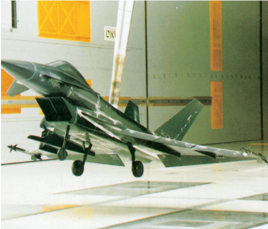
Model of conceptual European fighter undergoing tests in the German/Dutch (DNW) wind tunnel.
