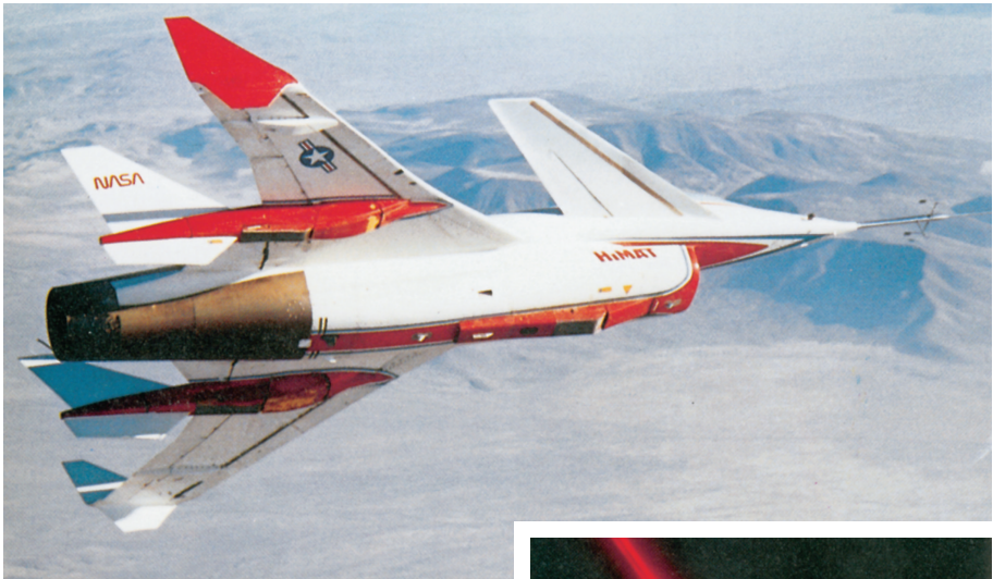
Guidance and control were important features of HIMAT, a remotely piloted research vehicle developed by NASA to investigate unusual and hazardous flight régimes.
