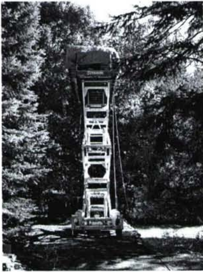
Fig. 1. This figure shows the lift with the experiment. The antennas are at the far end of the lift from the viewer under the roof that was built to shield the equipment from the elements. This picture was taken in September with the foliage largely still present. The cables coming from the lift are a ground cable to an earth ground and one of 4 tethers used in windy conditions.
