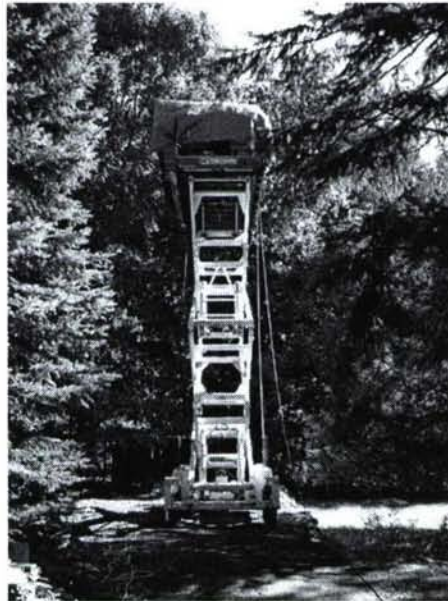
Figure 5: This figure shows the lift with the experiment. The antennas are at the far end of the lift from the viewer under the roof that was built to shield the equipment from the elements. This picture was taken in September with the foliage largely still present. The cables coming from the lift are a ground cable to an earth ground and one of 4 tethers used in windy conditions.
