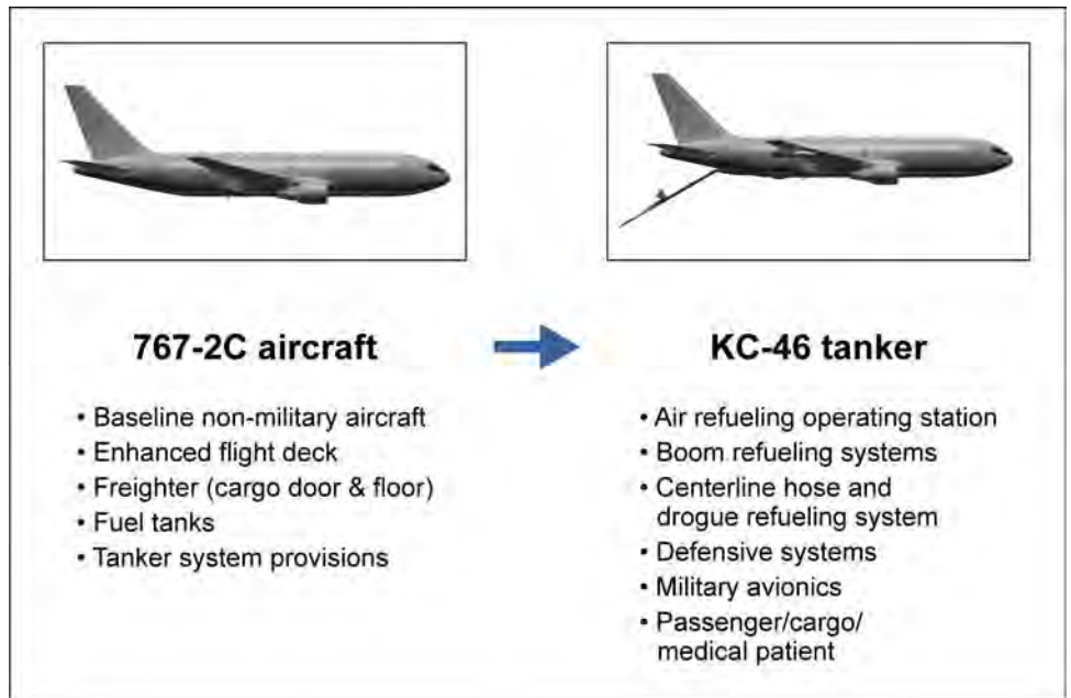
Figure 2: Conversion of Boeing 767-2C into KC-46 Aerial Refueling Tanker
