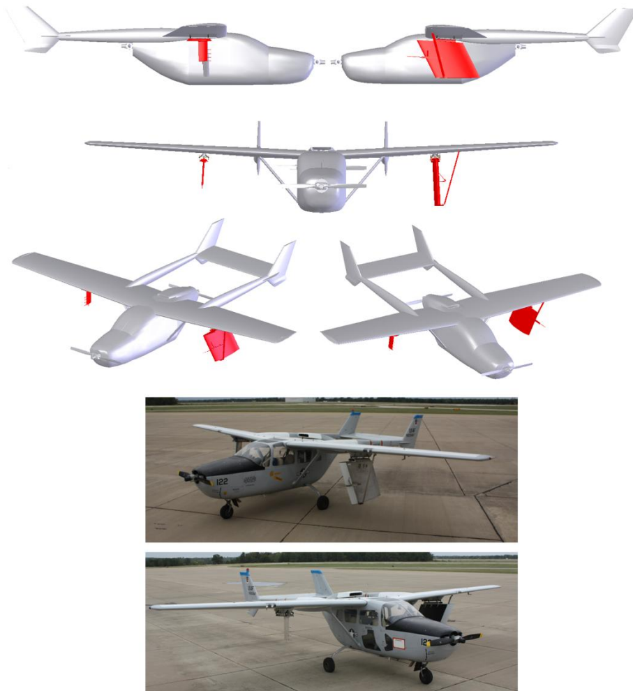
Figure 2: Cessna O-2A aircraft with SWIFT model and hotwire sting
