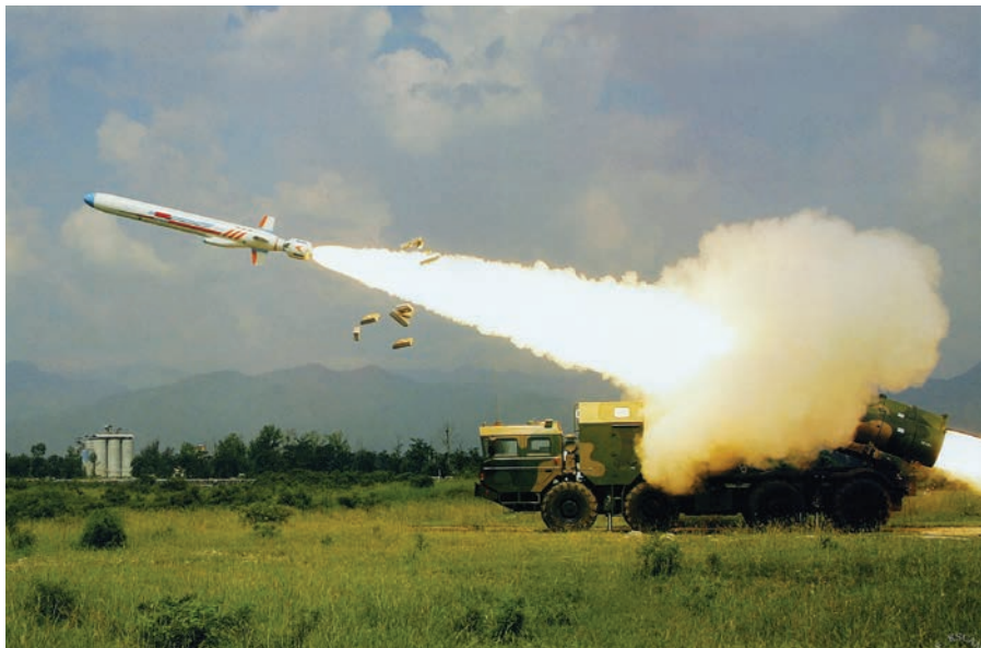
YJ-62 ASCM being launched by transporter erector launcher
