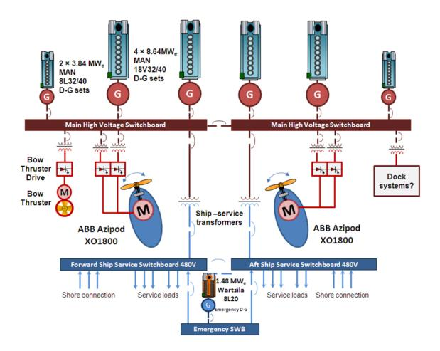
Figure 7: HSR(R) Machinery Schematic
