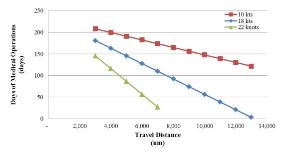
Figure 10: Predicted Unrefueled Maximum Time on Station (impact of transit to station)
