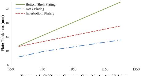
Figure 11: Stiffener Spacing Sensitivity Amidships
