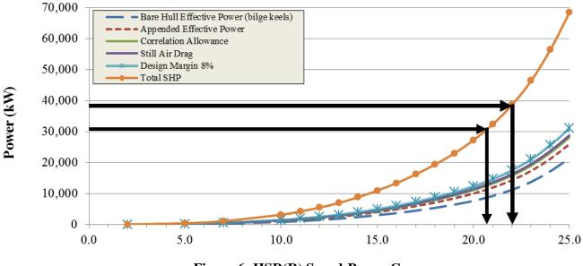
Figure 6: HSR(R) Speed-Power Curve
