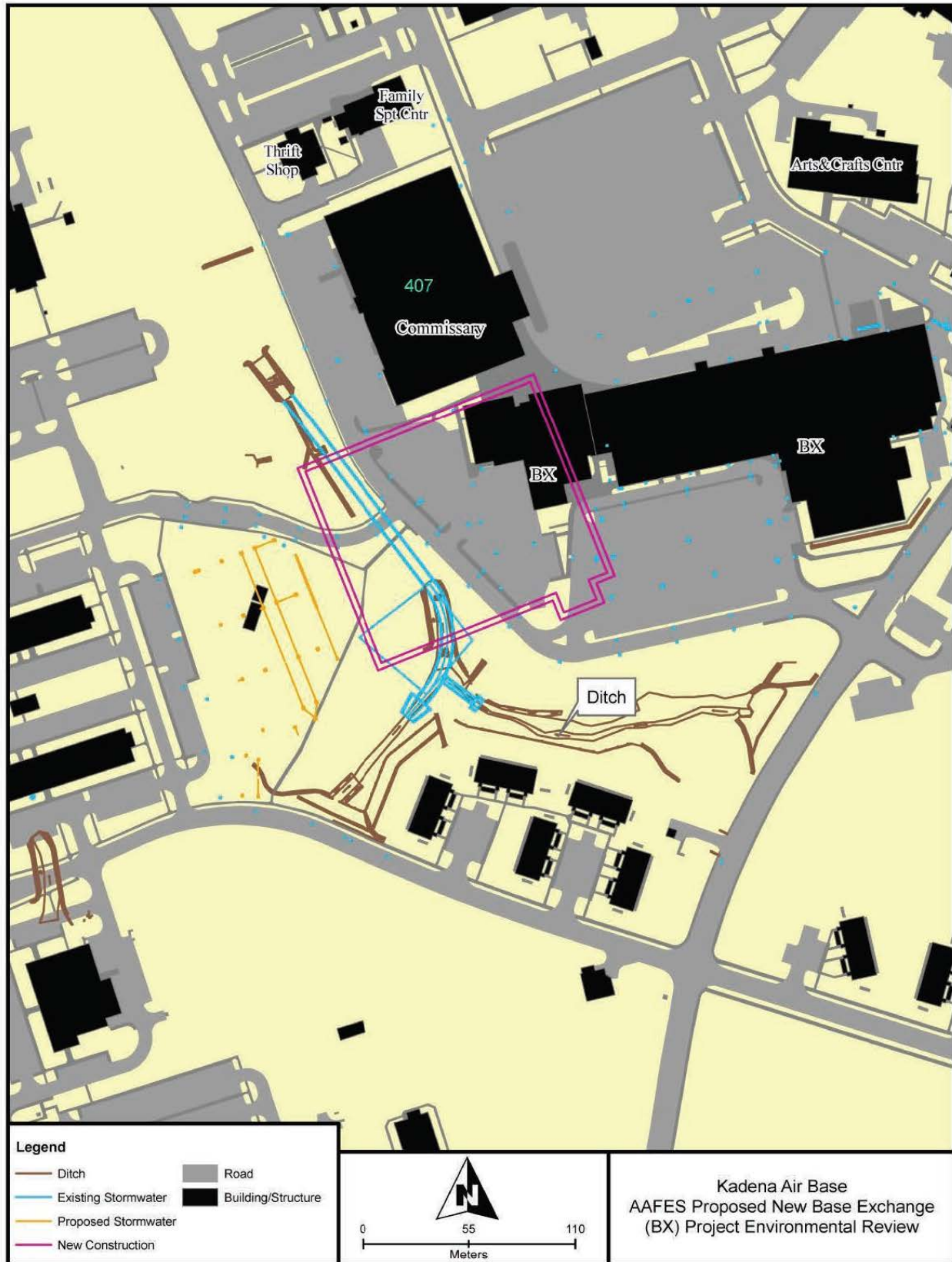
Figure 3-1. Stormwater System Within the Project Area
