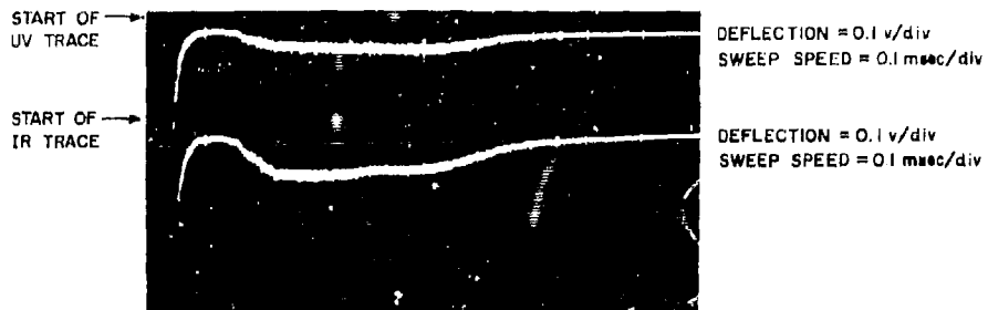
Fig. 15 - UV & IR Light Output Traces (Unintegrated) of the M6 Blasting Cap Illustrating the Primary and Secondary Reactions
