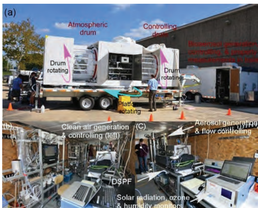
Fig. 6. A system, which was developed to study the transformation of optical properties and viability of bioaerosols exposed to different atmospheric environments, was carried out a field measurements at the High-Bay, ARL during September 27th through October 19th.
