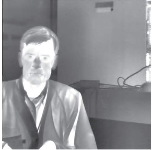
Fig. 10. Shows a 1-megapixel infrared image taken by an LC9 FPA at T = 52 K, -1 V and \tau_{\text{int}} = 2.0 ms.
