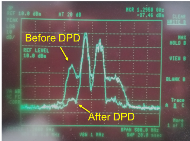
Fig. 10. Measured spectra of L2/L5 composite signal before and after DPD.
